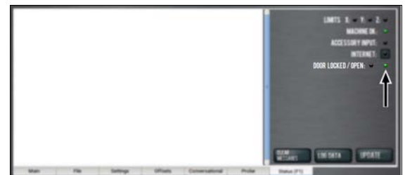
Figure 2-18: Door Open LED on the Status tab.
