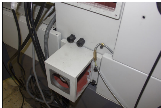
Figure 4-19: Cable glands installed.
