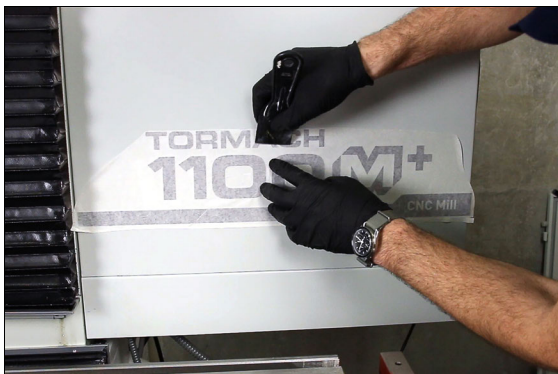
Figure 4-25: Pushing out air bubbles on the new decal.
