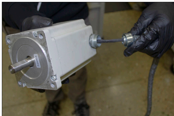
Figure 3-18: Removing the flex conduit from the X-axis motor.
