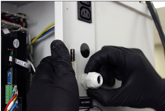
Figure 4-21: Securing the cord grip on the machine column.
