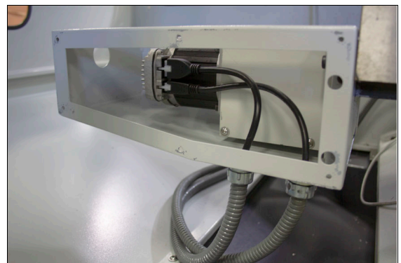
Figure 4-11: Wire connections on the X-axis motor.
