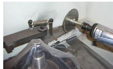
7. Clean all abrasive grit. Don't just brush it out. Vacuum it clean with a shop vac. Wipe everything down with an oiled cloth before reassembly. The photo at right shows the completed cut and cleaned cabinet.
