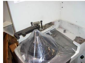
6. Make the cut. The photo shows the use of a hand held die grinder. We find the cut may take 10 minutes with a small pneumatic die grinder. An electric angle grinder takes about 60 seconds to make the cut. You will be trimming off about 0.1" to 0.3" of iron. The casting is about 0.7" thick at this point.
