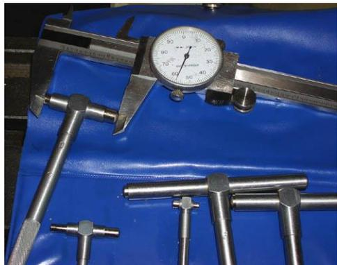
Figure 1 -Telescoping Gage
