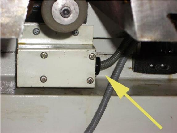
**Figure 2 – Cable without drip leg**
