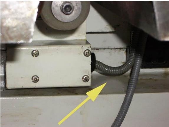
**Figure 3 - Cable with drip leg**
