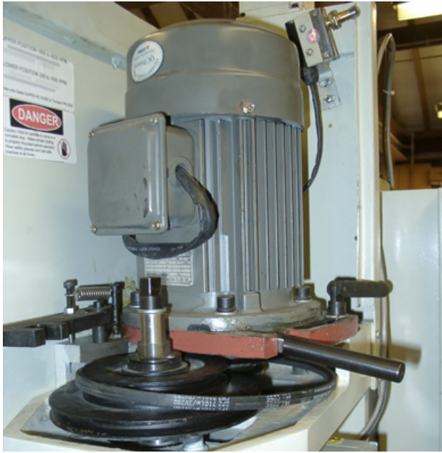
Figure 5.8: Changing Spindle Speed Range
