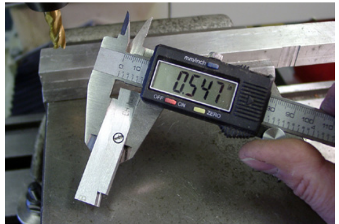
Figure 6.15: Measuring the Parallel Gauge
