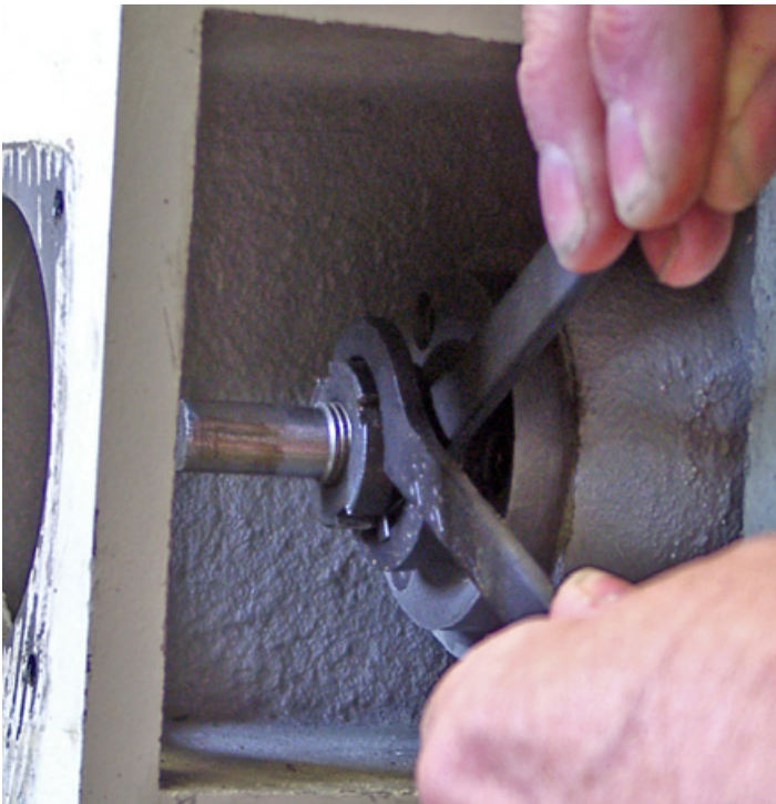
Figure 9.7: Tightening the lock nut.
