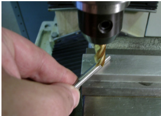
Figure 6.13: Gauge Just Rolls Under Tool
