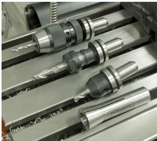
Figure 5.2: Holders in the TTS Range with Collet
