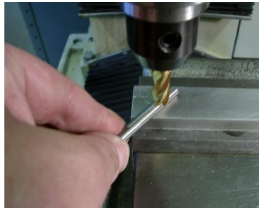
Figure 6.5 – Gauge just rolls under tool
