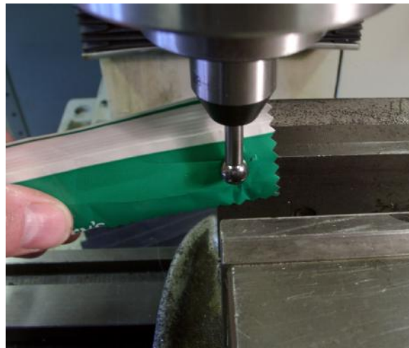
Figure 6.12 – Measuring vise jaw Y position
