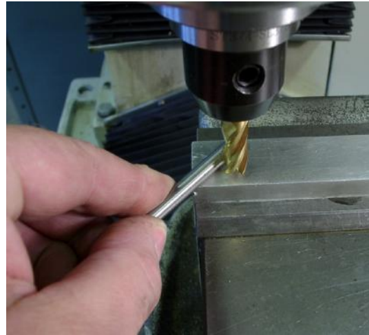
Figure 6.4 – Tool much too low for gauge
