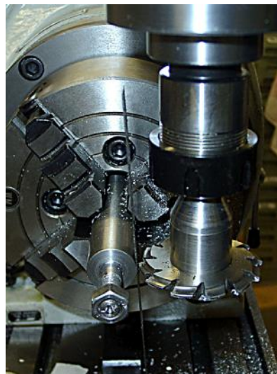
Figure 8.6 – Ruler tilted to left at top so cutter is too high
