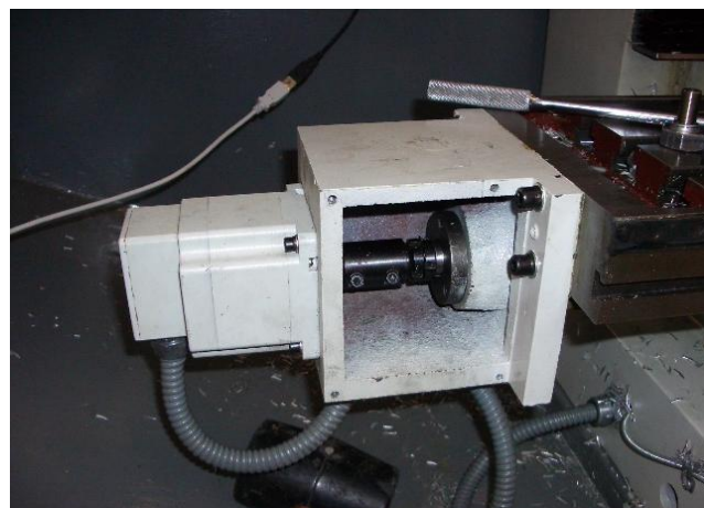
Figure 9.2 – Photograph of X-axis mount
