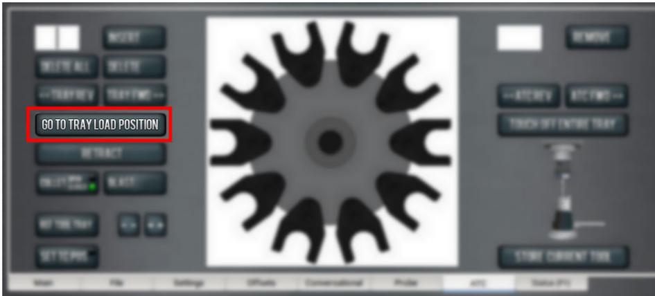
Figure 35: Go to Tray Load Position button on the ATC tab.
