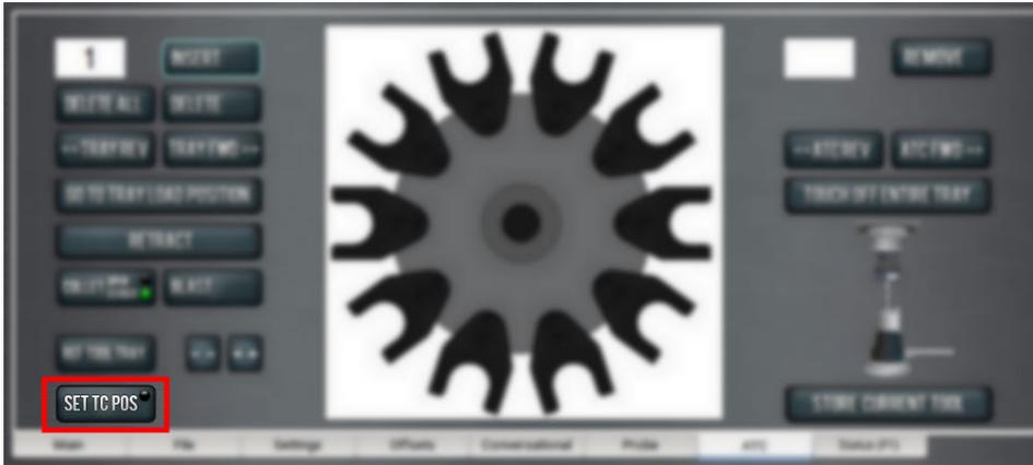
Figure 38: Set TC POS button on the ATC tab.
