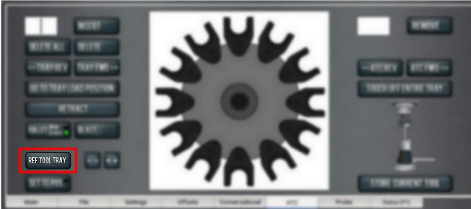
Figure 34: Ref Tool Tray button on the ATC tab.
