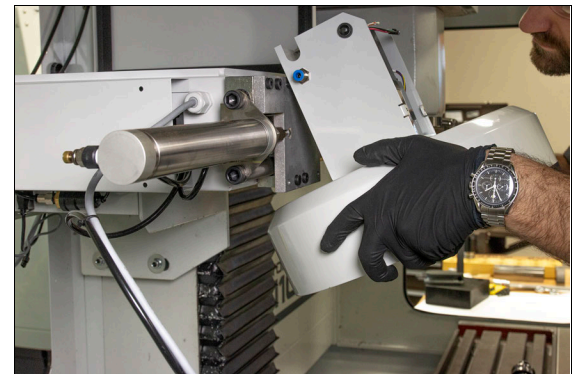
Figure 2-3: Hanging the ATC onto the actuator plate.
