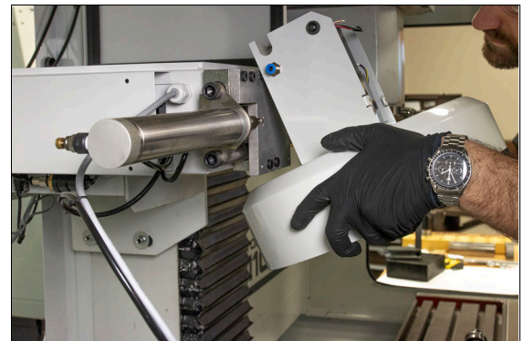
Figure 2-3: Hanging the ATC onto the actuator plate.
