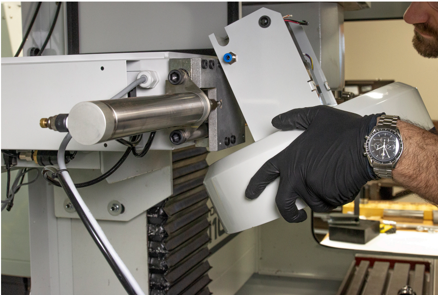
Figure 3: Hanging the ATC onto the actuator plate.
