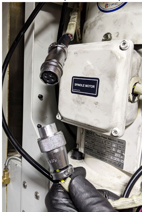
Figure 1: Spindle motor quick-connect fitting disconnected.
