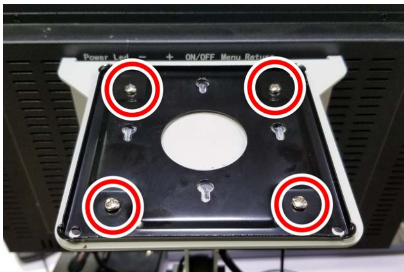
Figure 2: VESA plate mounted onto the PathPilot Controller VESA Mount (PN 50382) .
