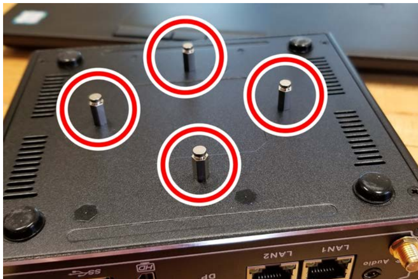
Figure 1: Installing the standoffs on the controller.
