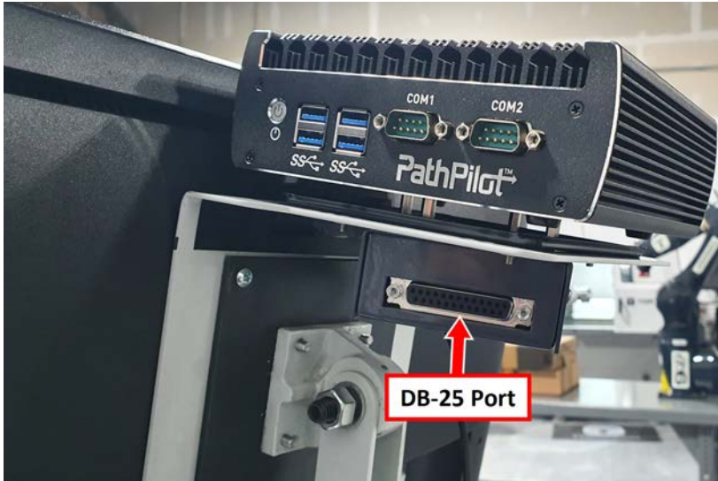
Figure 5: Adapter attached to the bottom of the mount.
