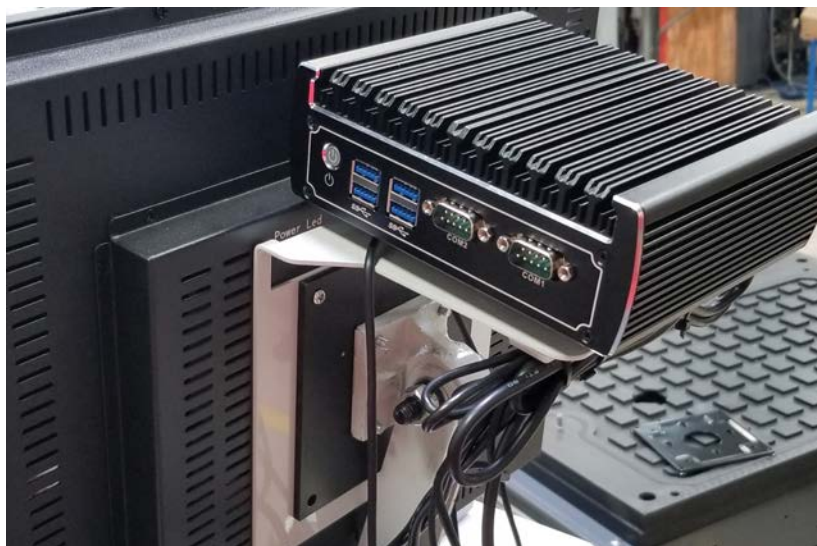
Figure 3: Controller attached to the top of the mount.
