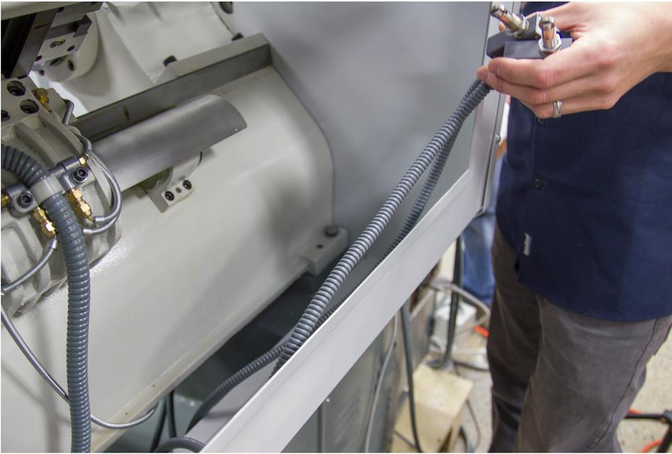
*Figure 2: Door switch cables routed to the front of the machine.*
