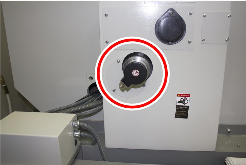
*Figure 3: Rotary encoder on the belt guard cover.*
