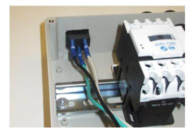
Next you need to install the coil wires. The white wire will go to AI and the black wire goes to A2.
