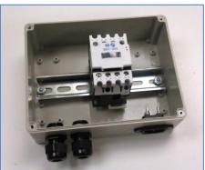
With the DIN rail installed, you can snap the relay contactor onto the DIN rail.
