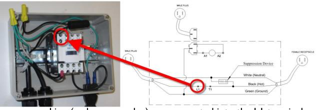
Line (male power plug) are connected into the LI terminal
