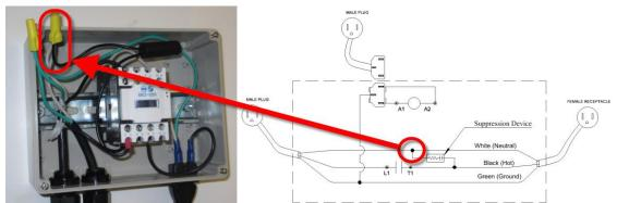
Neutrals from both Load and Line are connected to suppression device with a wire nut. The neutral wires are the white wires.
