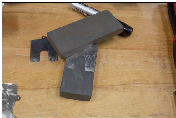
Figure 2-11: Shim stock between two machinist stones.
