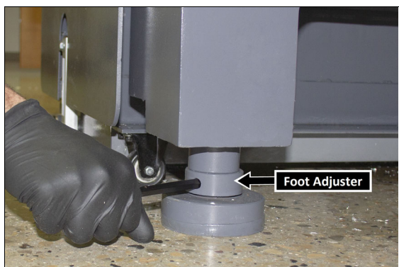
Figure 2-6: Adjusting the machine stand's feet on a 770M.
