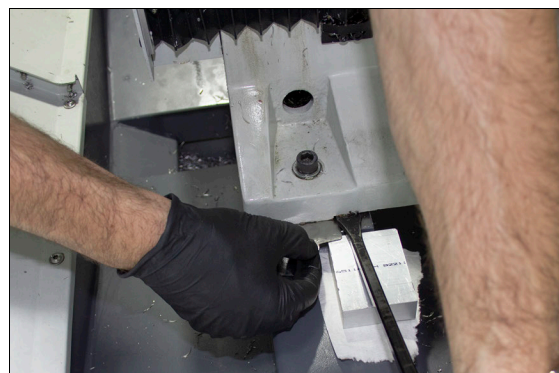
Figure 2-15: Putting a shim stock piece between the base and the stand.
