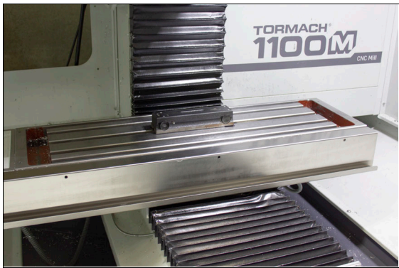
Figure 2-9: Machine table moved to the Y- limit.
