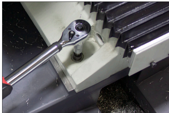
Figure 2-12: Loosening the front bolt on the base.
