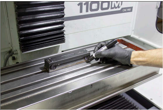
Figure 2-4: Marking the location of the precision level on the machine table.
