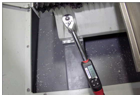
Figure 2-16: Tightening the front bolt on the base.
