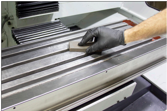
Figure 2-1: Removing burrs from the machine table.
