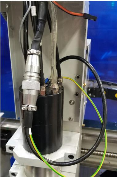
*Figure 11: Spindle power connector.*
