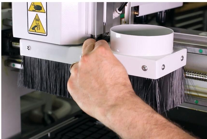
*Figure 51: Pressing down on the dust shoe.*
