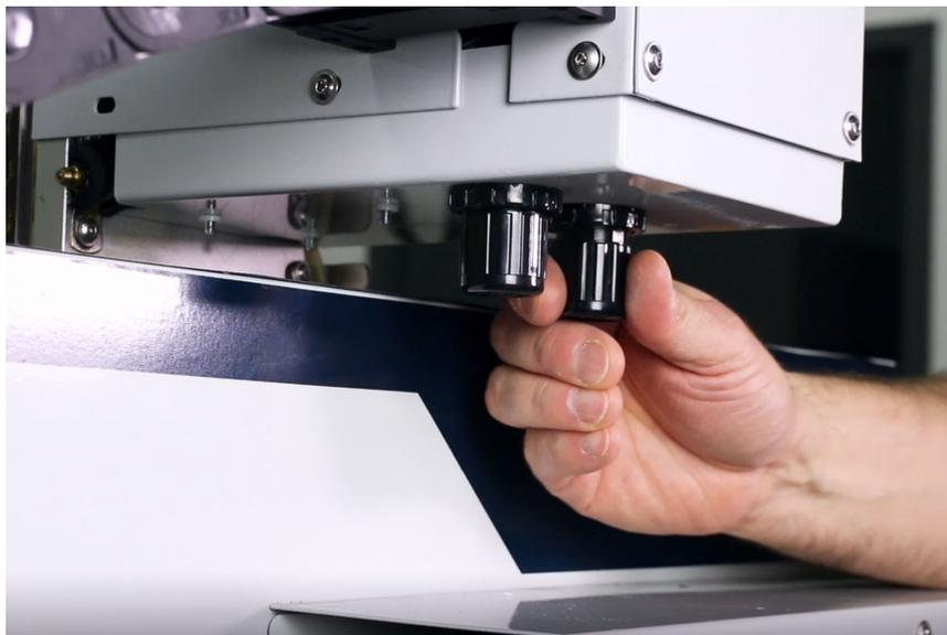
*Figure 48: Unlocking the dust shoe extend pressure regulator.*
