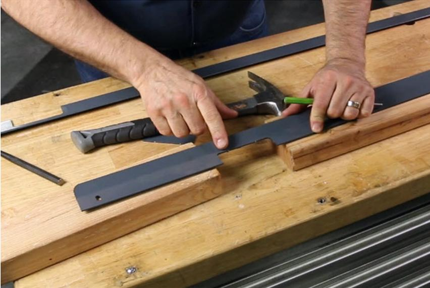
*Figure 42: Linear rail cover with punch-out removed.*
