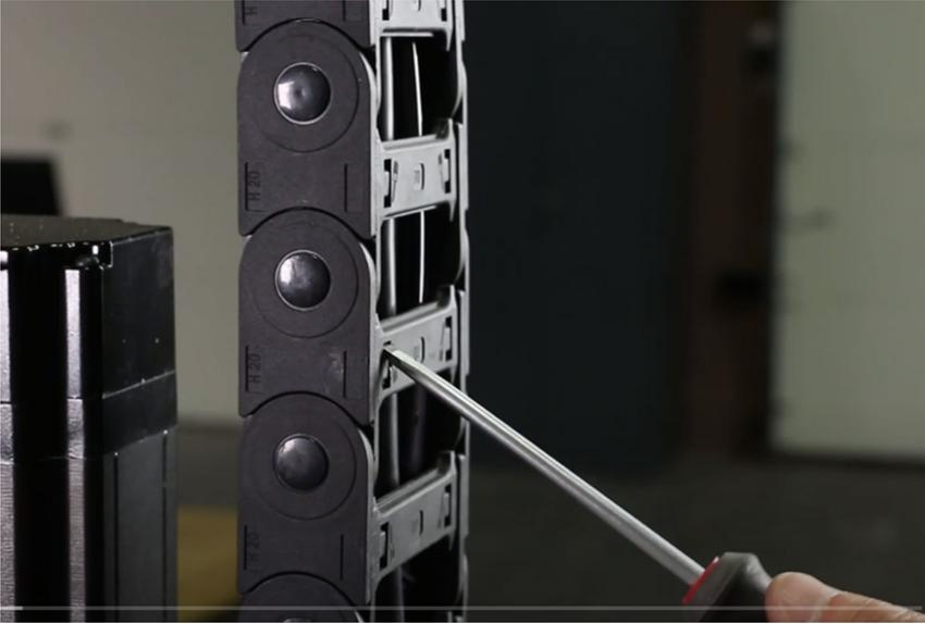
*Figure 12: Removing pieces of the energy chain.*
