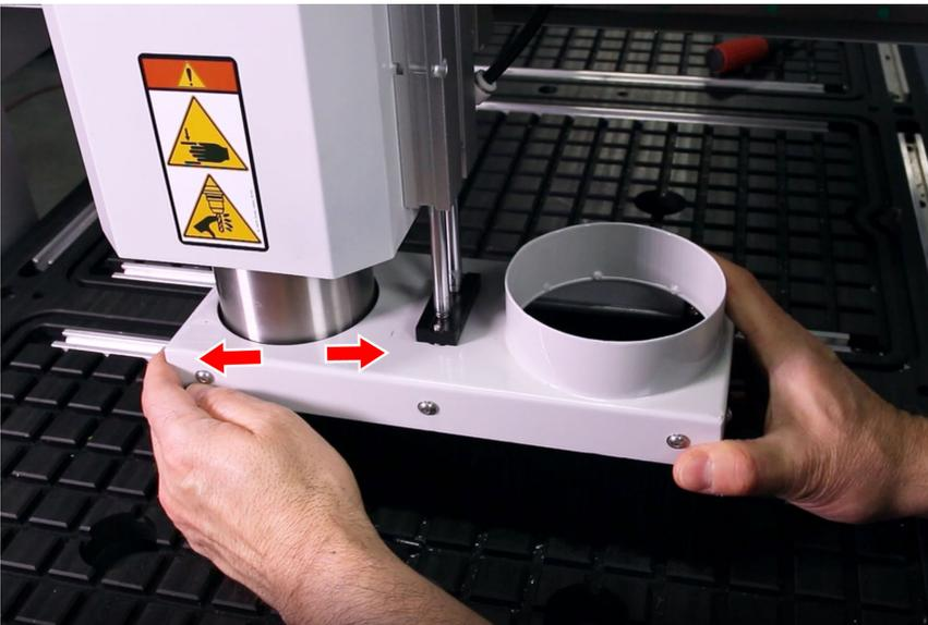
*Figure 33: Adjusting the position of the dust shoe.*
