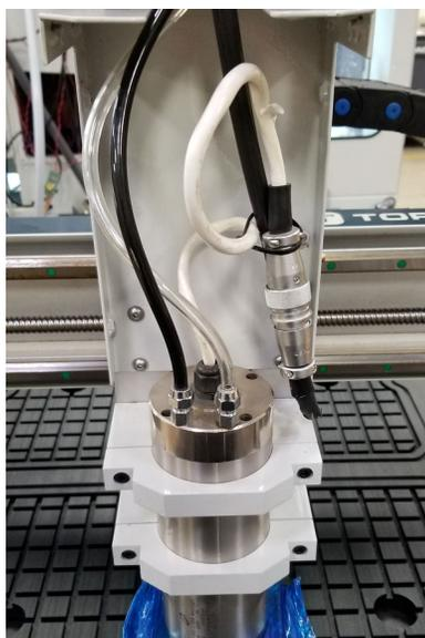
*Figure 3: Spindle power connector.*
