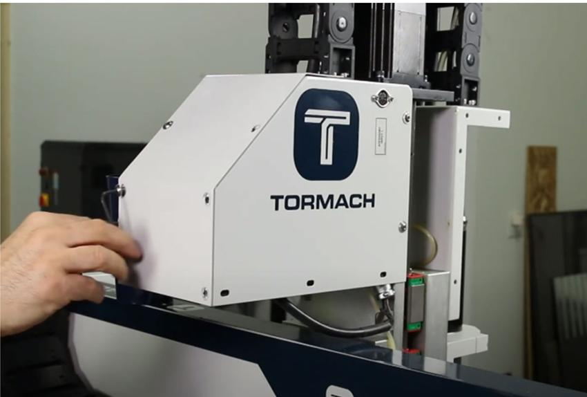
*Figure 13: Rear Z-axis access panel.*
