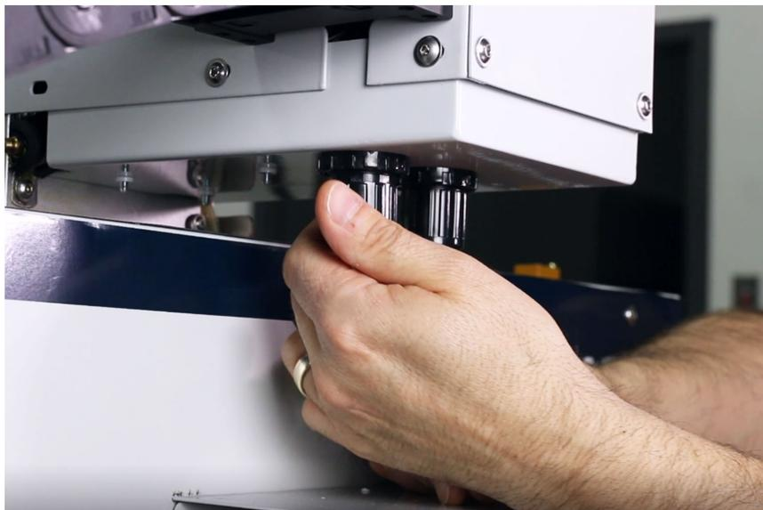
*Figure 50: Unlocking the dust shoe lift pressure regulator.*
