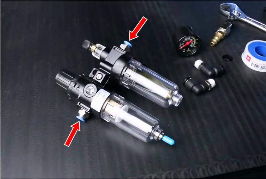
*Figure 22: Preinstalled push-to-connect fittings on the FRL.*
