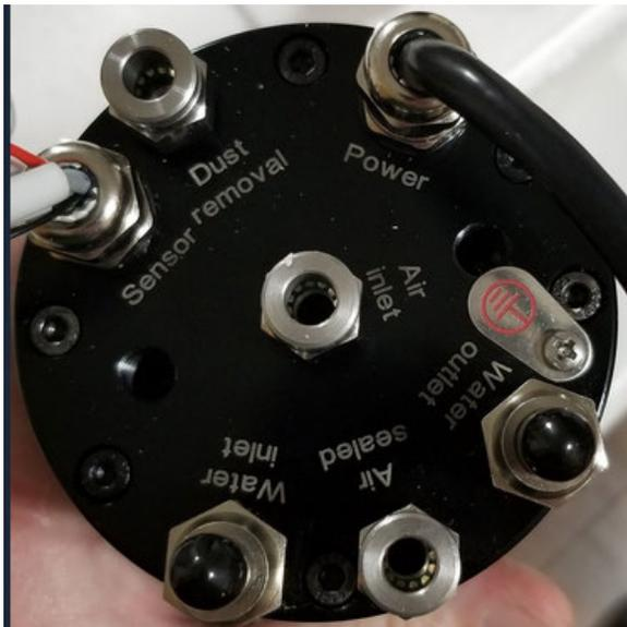
Figure 28: Air line connections.
