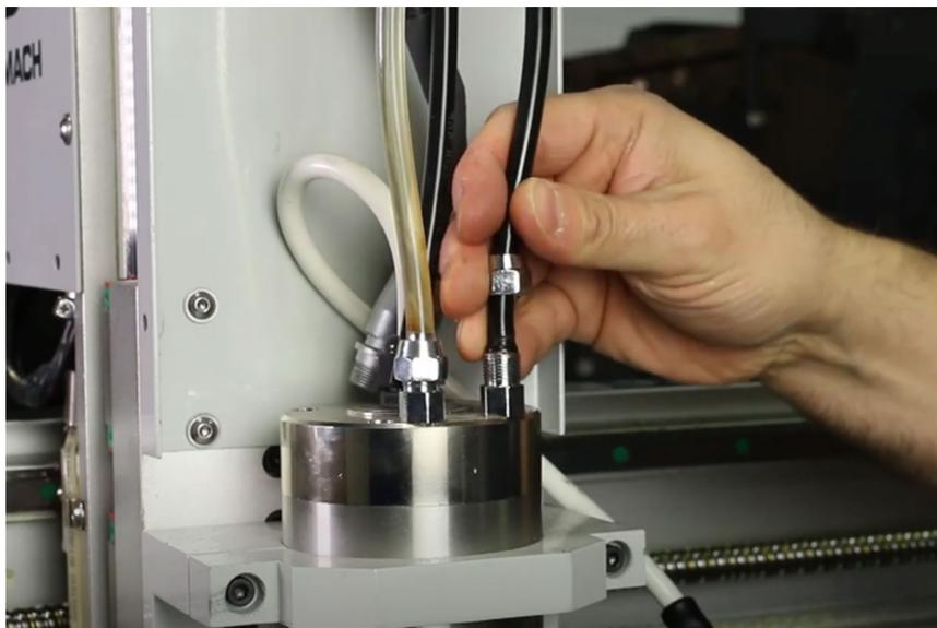
*Figure 4: Two water lines on the existing spindle.*
