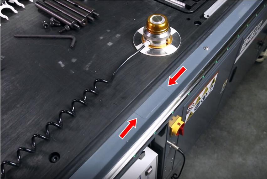
Figure 39: Linear rail cover punch-outs.
