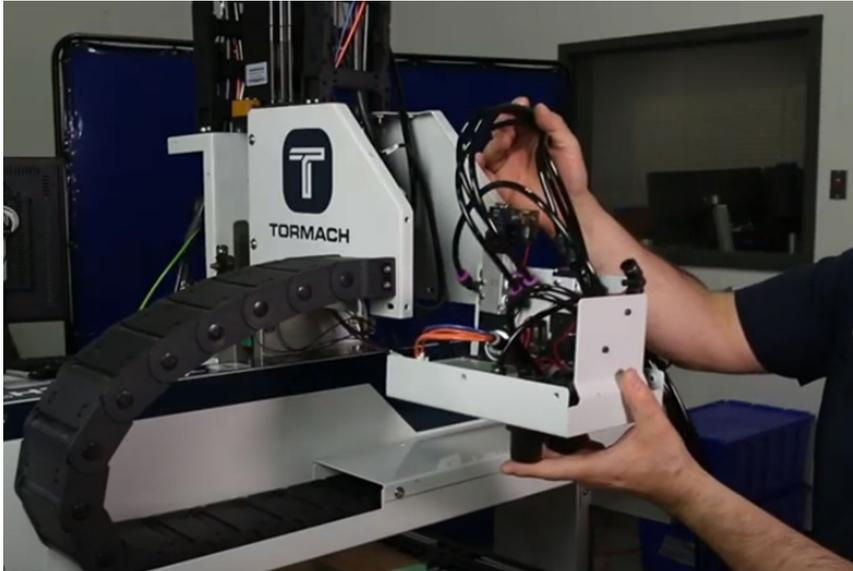
*Figure 21: Solenoid control assembly.*
