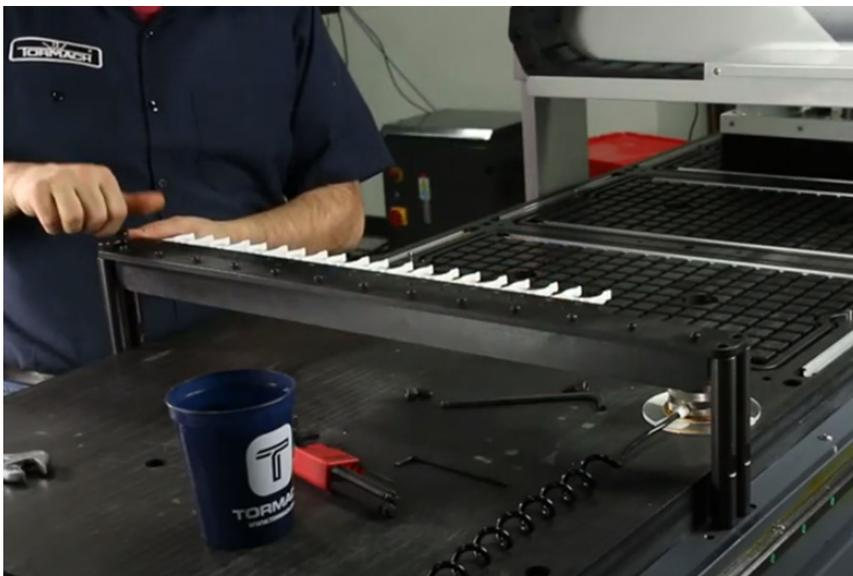
Figure 45: Installing the rack onto the standoffs.
