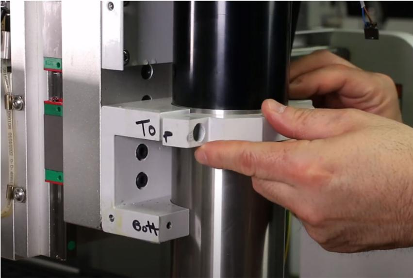
*Figure 8: Mounting the ISO20 spindle.*
