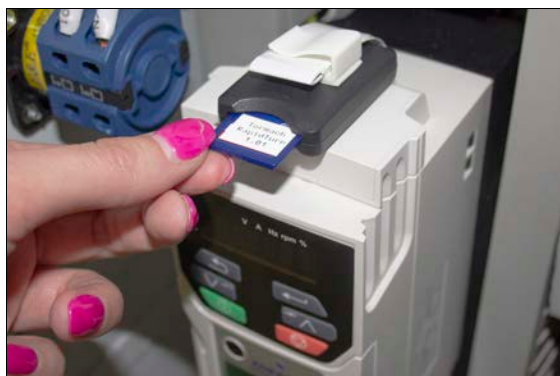
Figure 3-1: Tormach High Speed Spindle SD Card inserted into the VFD.
