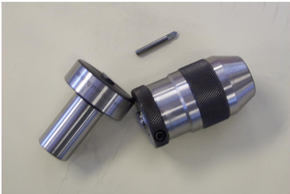
Figure 1: Jacobs taper adapter and drill chuck.
