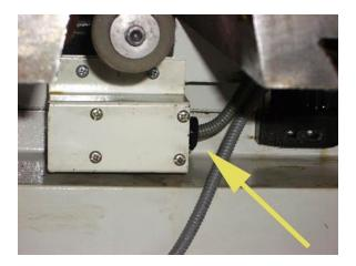
Figure 2 – Cable without drip leg
