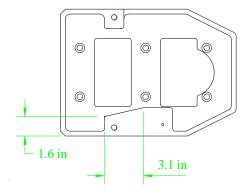
Figure 5 – Motor Base Dimension
