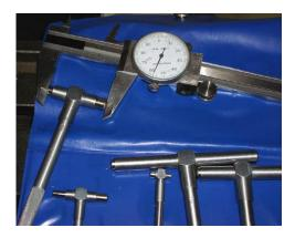
Figure 1 -Telescoping Gage
