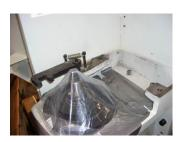
6. Make the cut. The photo shows the use of a hand held die grinder. We find the cut may take 10 minutes with a small pneumatic die grinder. An electric angle grinder takes about 60 seconds to make the cut. You will be trimming off about 0.1" to 0.3" of iron. The casting is about 0.7" thick at this point.
