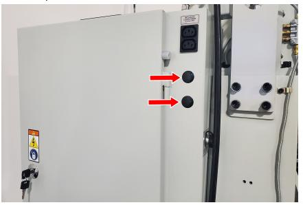
Figure 1: Knockout holes on the machine column.
