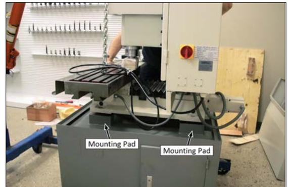
**WARNING!** Crush Hazard: While lowering the machine onto the Machine Stand, you must keep your hands away from all moving parts.
