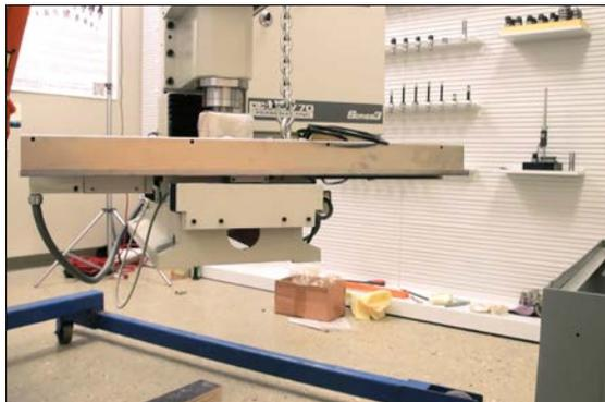
If necessary, lower the machine and, from the machine table, adjust the position of the M12 T-nuts.
