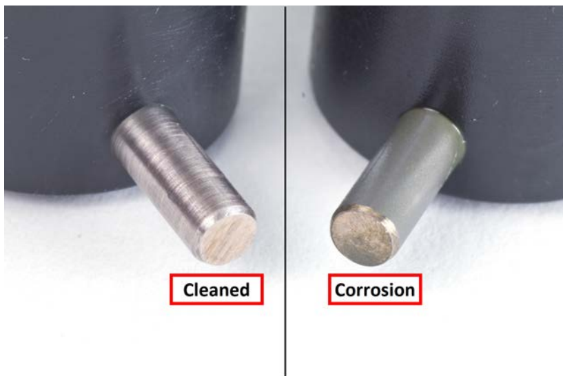
Figure 4: Example of a cleaned contact spoke next to a contact spoke with corrosion.
