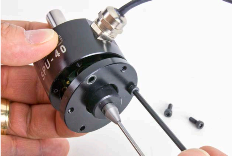
Figure 1: Removing the screws from the probe.
