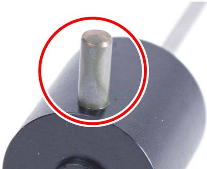
Figure 3: Example of corrosion on a contact spoke.
