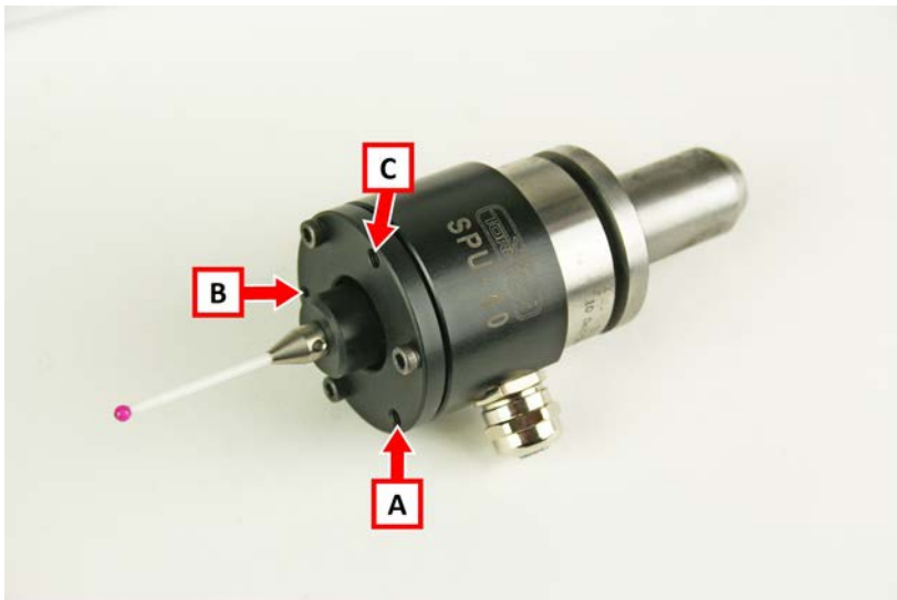
Figure 2: Adjustment set screws on the probe.
