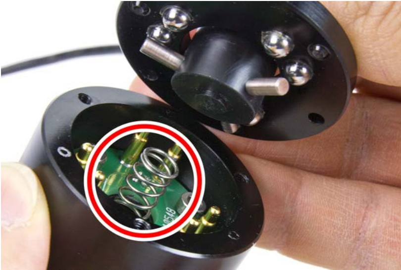
Figure 5: Spring aligned correctly in the probe.
