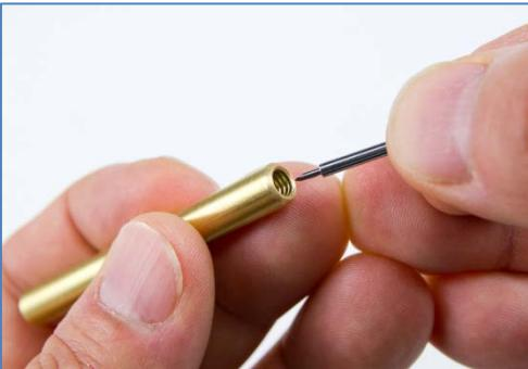
4. Place the cone-shaped end of the replacement blade (opposite the knife end) into the center hole of the external ball bearing and push the ball bearing into the brass housing until it is flush with the end of the housing.
