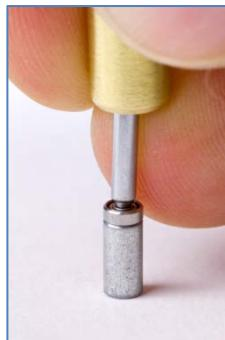
6. Tilt the brass housing slightly to the left or right, and use the tip of one finger to hold the steel spacer in place.
