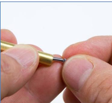
5. Insert the steel spacer into the brass housing in a similar manner and push the end of spacer into the brass housing until it is flush with the end of the housing.
