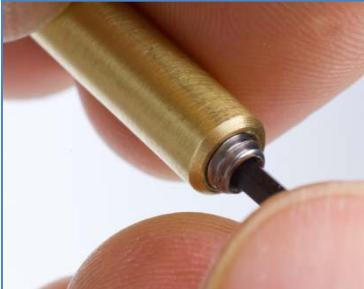
2. Turn the wrench counter-clockwise to completely remove the setscrew.
