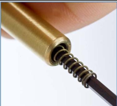
Note: If the bearing catches on the threads inside the brass housing, gently tap the protruding end of the hex wrench against the table or hard work surface.
