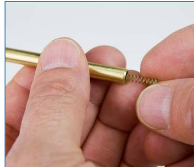
Note: If the spring does *not* slide freely into the brass housing, repeat steps 1-7 until the spring is in correct orientation.
