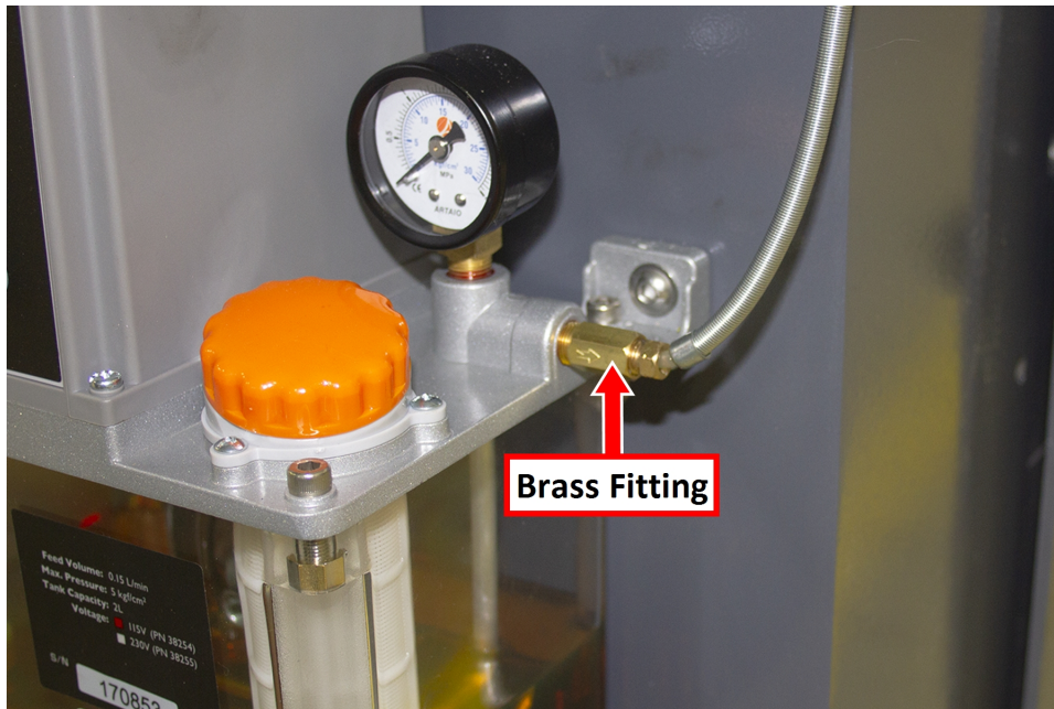
Figure 2: Brass fitting on the automatic oiler.
