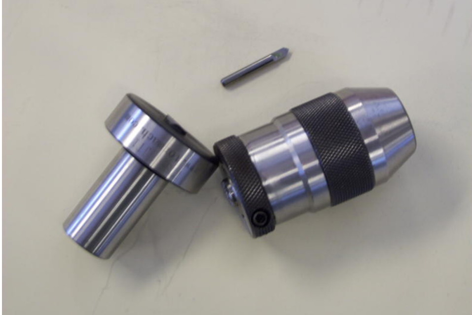
Figure 1: Jacobs taper adapter and drill chuck.
