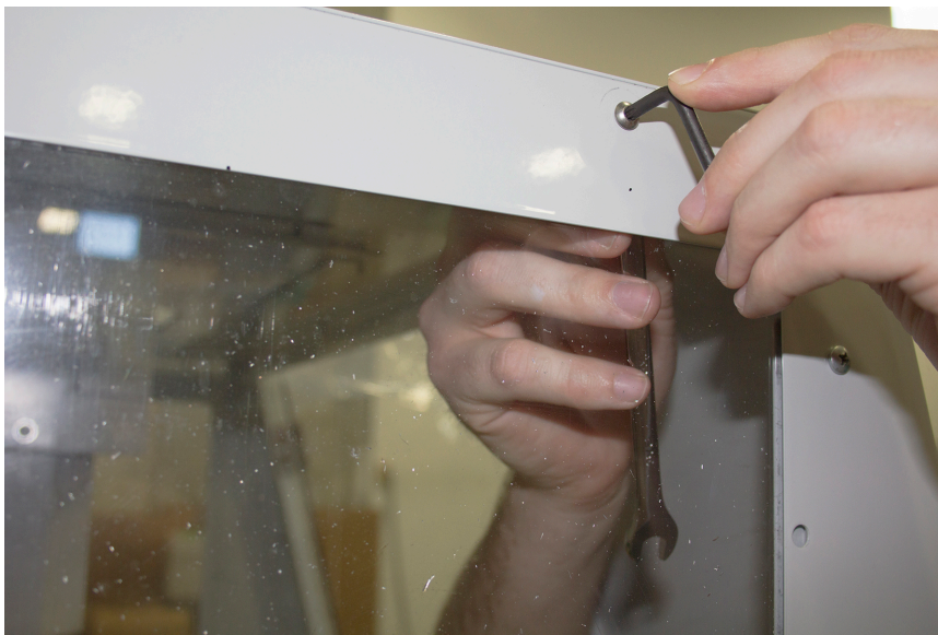
Figure 10: Example of securing a lock nut to a safety screw.
