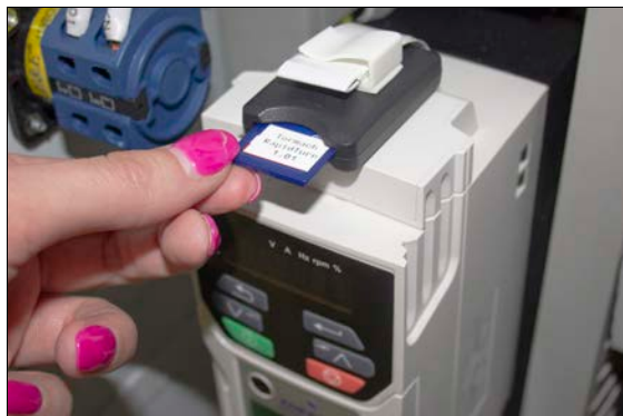
Figure 3-1: Tormach RapidTurn® SD Card inserted into the VFD.
