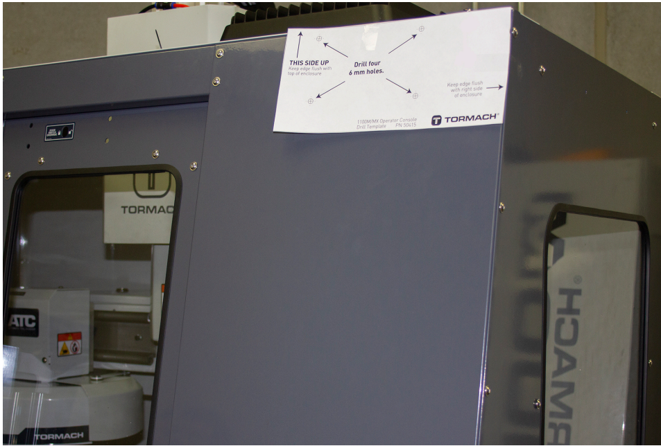
Figure 1: Drill template taped to the enclosure.
