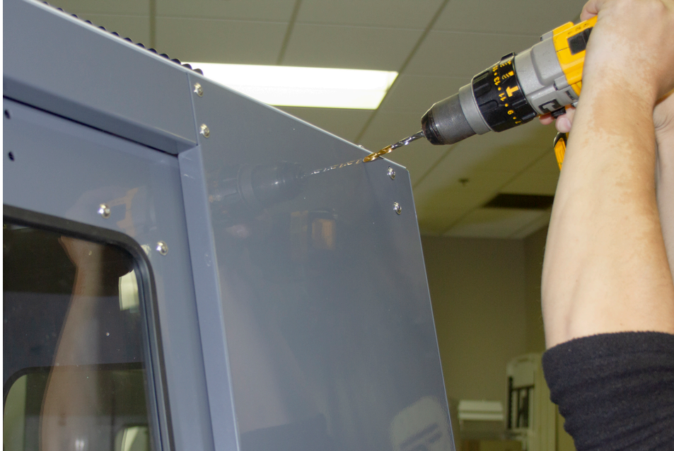
Figure 2: Drilling holes into the top of the enclosure.
