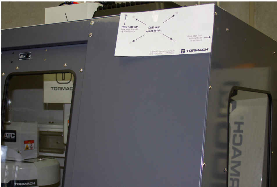
Figure 1: Drill template taped to the enclosure.
