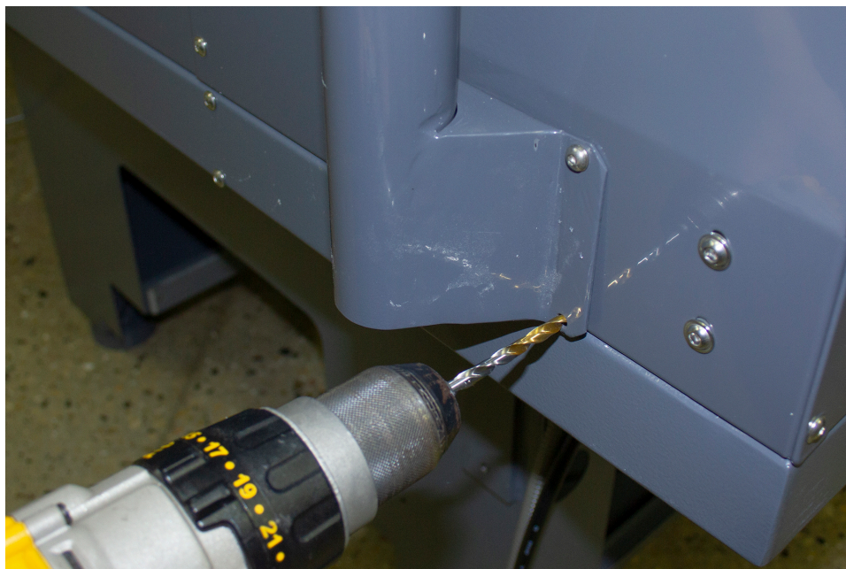
Figure 5: Drilling the remaining three holes into the enclosure.
