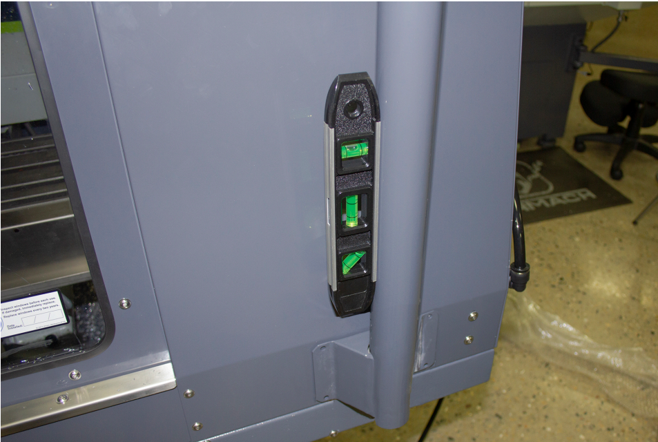
Figure 4: Bottom of the mount arm level on the enclosure.
