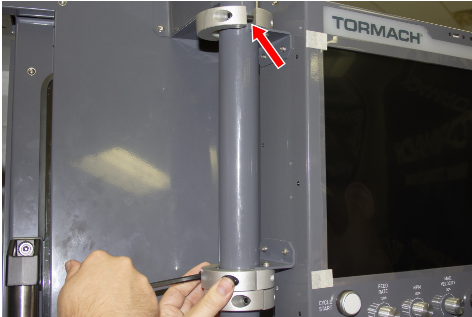
Figure 14: Loosely attaching the split collars to the mount arm.
