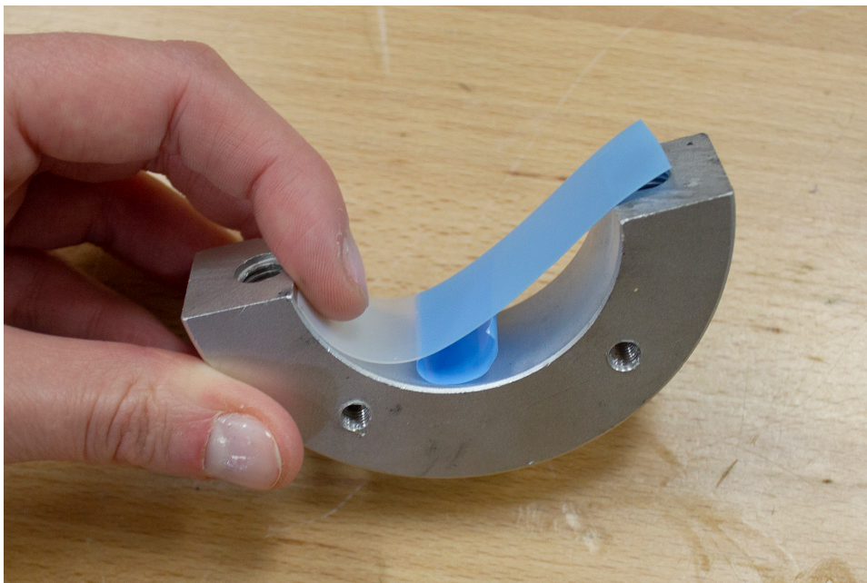
Figure 8: Adhering tape on the inside of a split collar.
