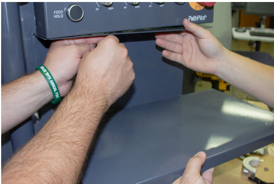
Figure 15: Attaching the keyboard tray to the bottom of the controller.
