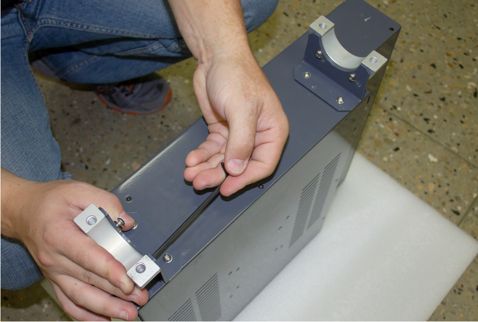
Figure 11: Split collars attached to the mount arm brackets on the controller.
