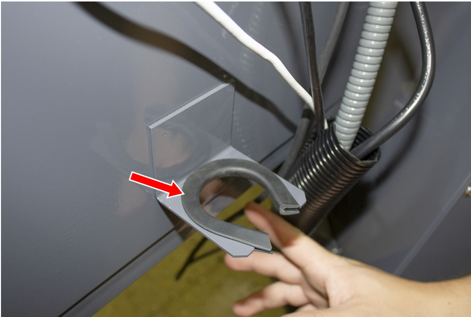
Figure 18: Rubber attached to the bracket on the keyboard tray.
