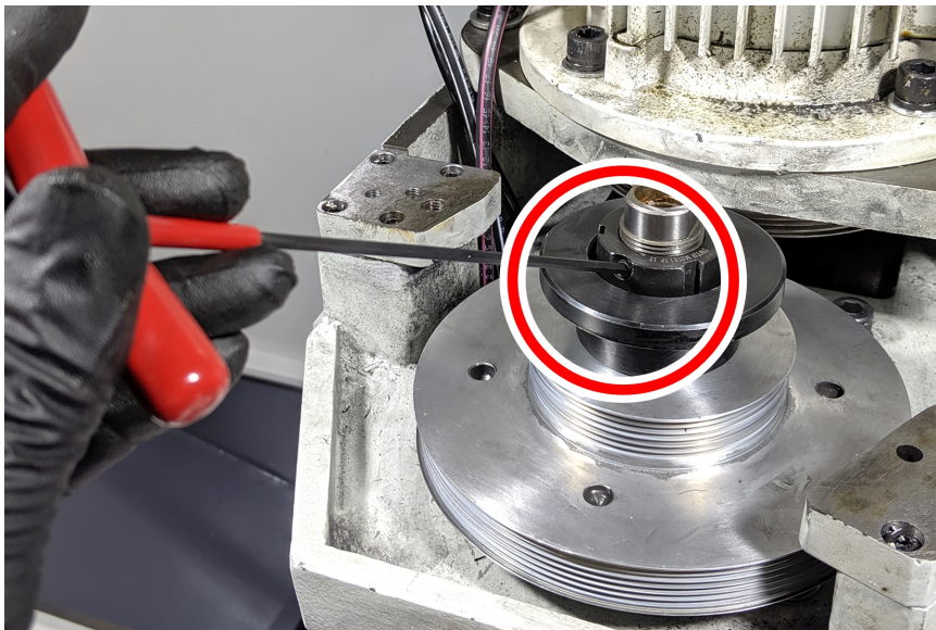
Figure 11: Loosening the retention nut's set screws.
