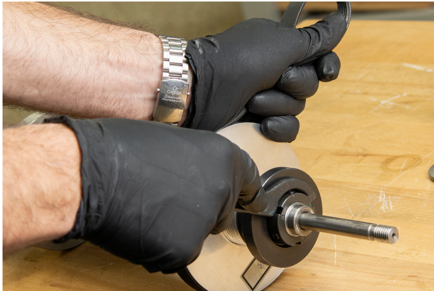
Figure 25: Removing the retention nut.
