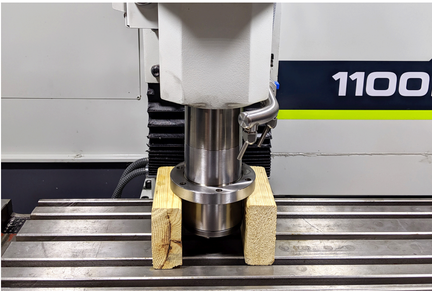
Figure 28: Z-axis jogged down to move the head casting over about half of the BT30 spindle.
