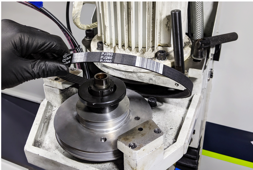
Figure 10: Removing the spindle belt.
