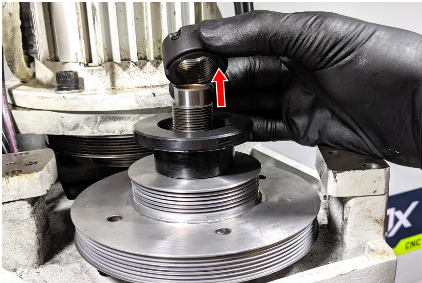
Figure 12: Removing the retention nut.
