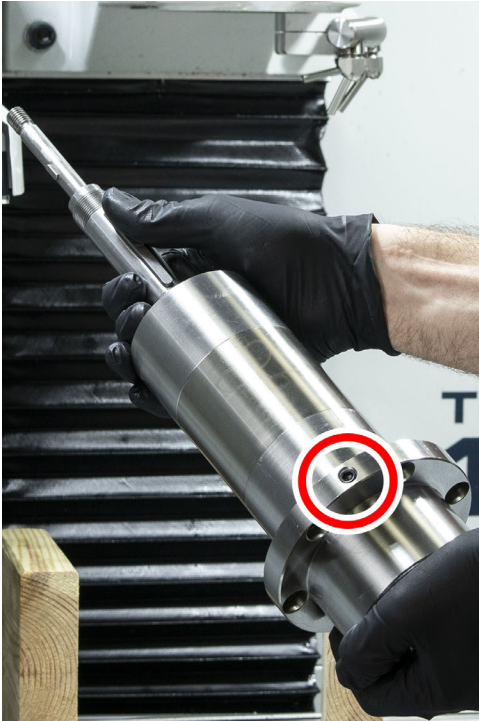
Figure 27: Hole on the spindle, which you must verify is pointing toward the machine column to install.
