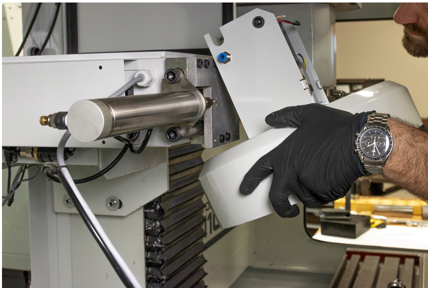
Figure 3: Hanging the ATC onto the actuator plate.
