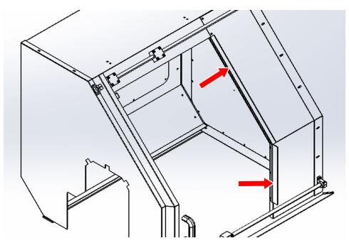
Figure 22: Door brush installed to the left side of the front right panel.
