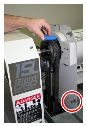
Figure 4: Lower right belt guard cover mounting bracket.
