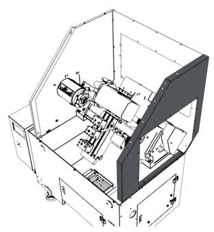
Figure 10: Right side panel installed.
