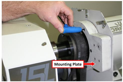
Figure 5: Loosening the socket head cap screw on the mounting plate.
