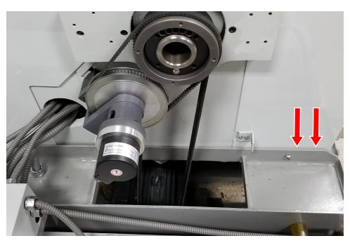
Figure 8: Correct position of the left side panel, which is inside of the machine stand.
