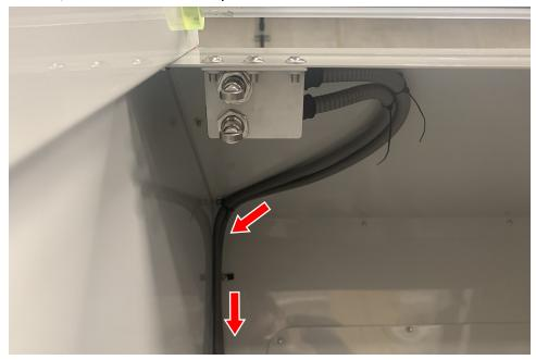
Figure 19: Door switch cable routing.
