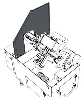
Figure 7: Left side panel installed between the mounting plate and the sheet metal guard.
