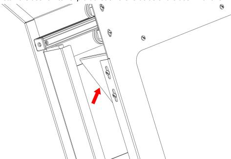
Figure 20: Door switch trip bracket installed.
