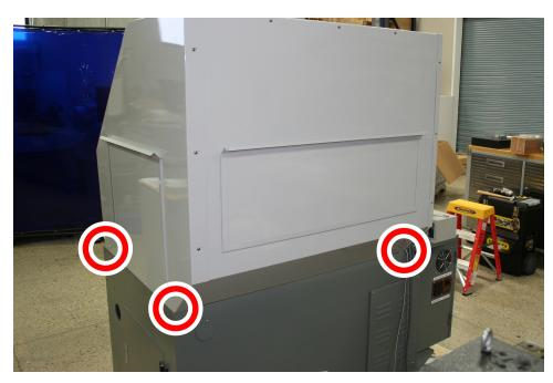
Figure 13: Corners on which to secure the enclosure to the machine stand.
