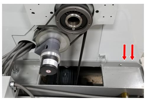
Figure 6: Left side panel installed between the mounting plate and the sheet metal guard.
