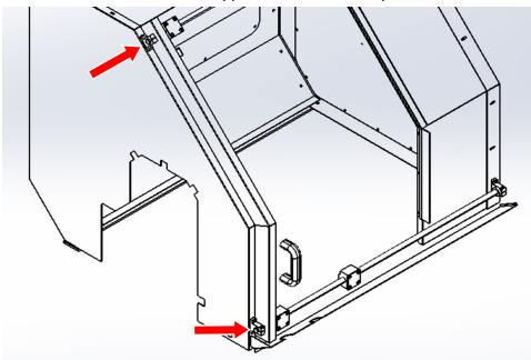
Figure 15: Linear rail supports attached to the left side panel.
