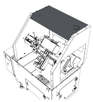
Figure 11: Top panel installed.
