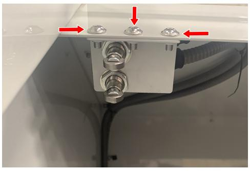
Figure 18: Door switch installed.
