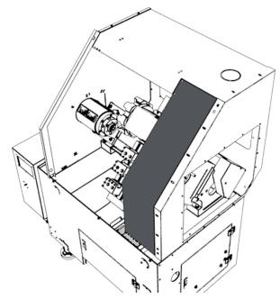
Figure 12: Front right panel installed.
