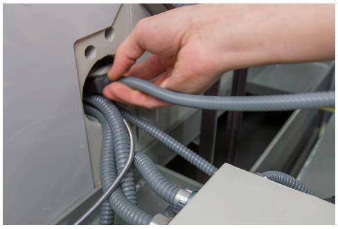
Figure 1: Routing the door switch cables through the base casting hole.
