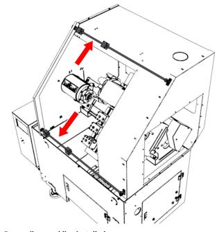
Figure 16: Door rail assemblies installed.
