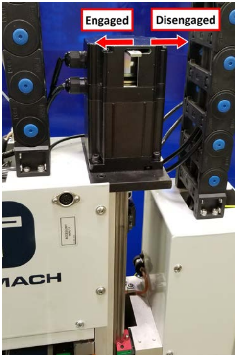
Figure 11: Replacement Z-axis motor installed onto the machine.
