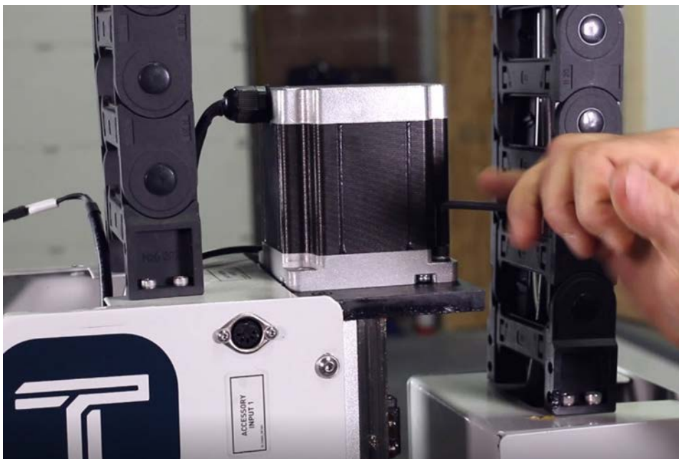
Figure 9: Existing Z-axis motor secured to the machine.
