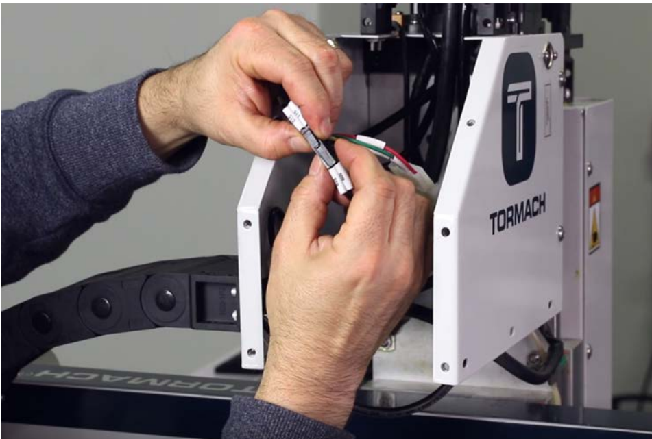
Figure 13: Connecting the Z-axis brake cable to the Z-axis motor's brake connector.
