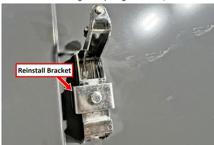
Figure 10: Attaching the door latch to the door with the bracket.
