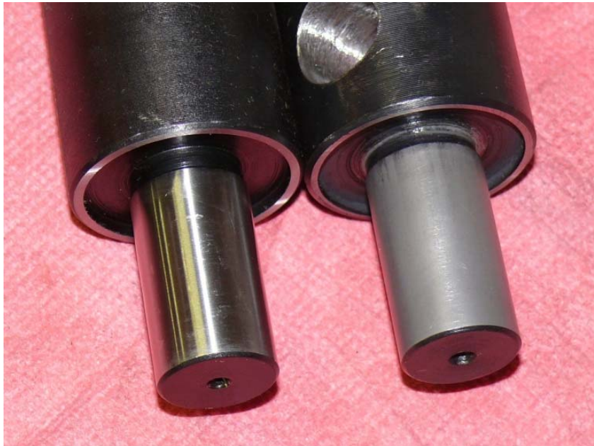
Figure 15 - Effect of 600 grit compound on shank after about 10 torque / failure cycles. New TTS blank on left for comparison
