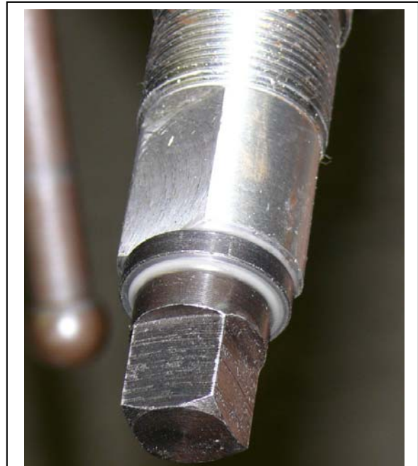
Figure 12 - Anti-seize applied between thrust washer and spindle.
