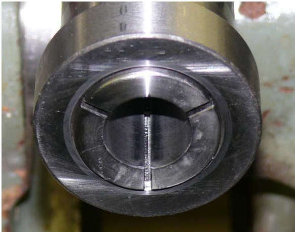
Figure 17 - Effect of 1200 grit compound on collet
