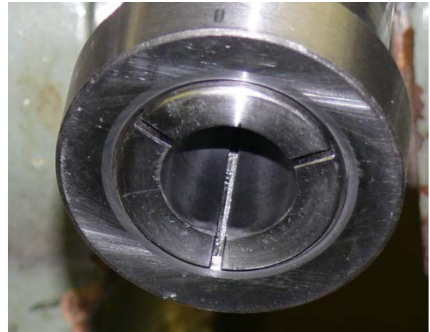
Figure 18 - Effect of 600 grit compound on collet
