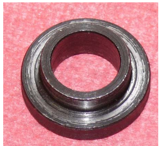
Figure 8 - Close View of Galled Washer
