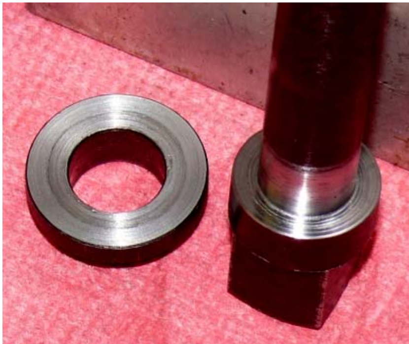
Figure 16 - Thrust surfaces after about 50 tests with anti-seize. Looks great and feels smooth.
