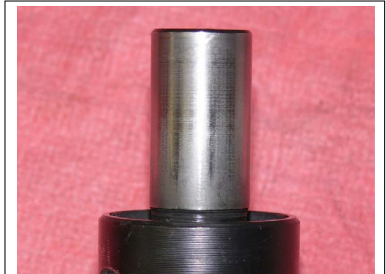
Figure 14 - Effect of 1200 grit compound on shank after about 10 torque / failure cycles
