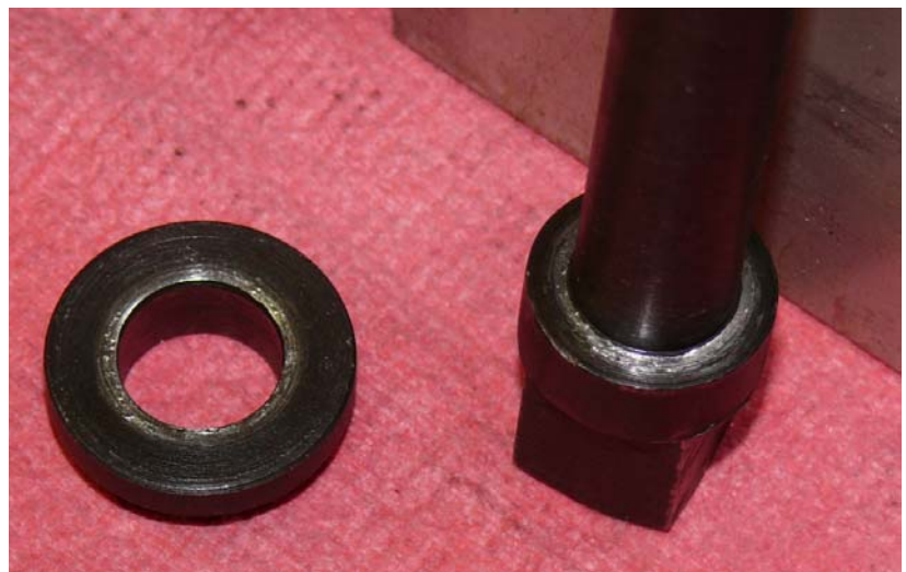
Figure 7 - Galled Thrust Washer and Drawbar
