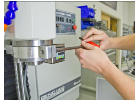
Figure 6. Tighten Hex nut to secure position
