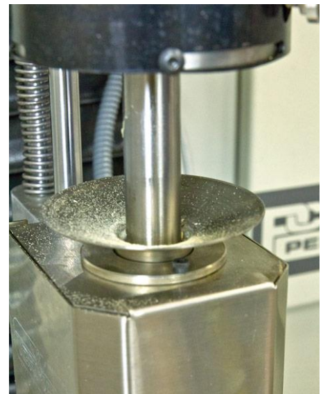
Figure 11. Ram should pass without issue. If severe interference exists, adjust ram position and/or heater box alignment.
