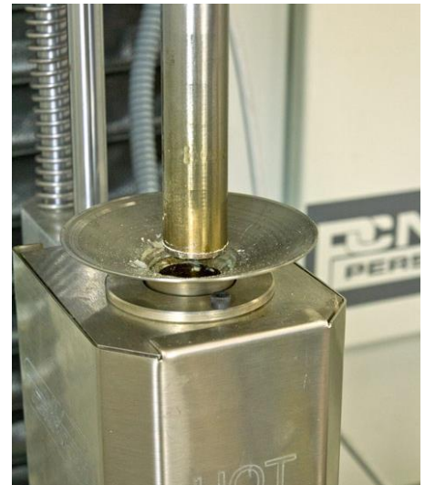
Figure 10. To check for interference, slowly jog ram into receiver.
