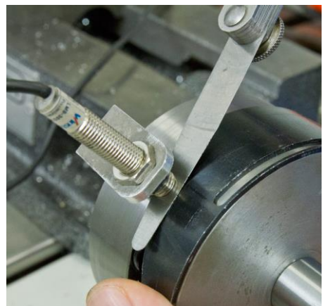
Figure 3. Adjust Sensor position; use feeler gauge or similar as reference
