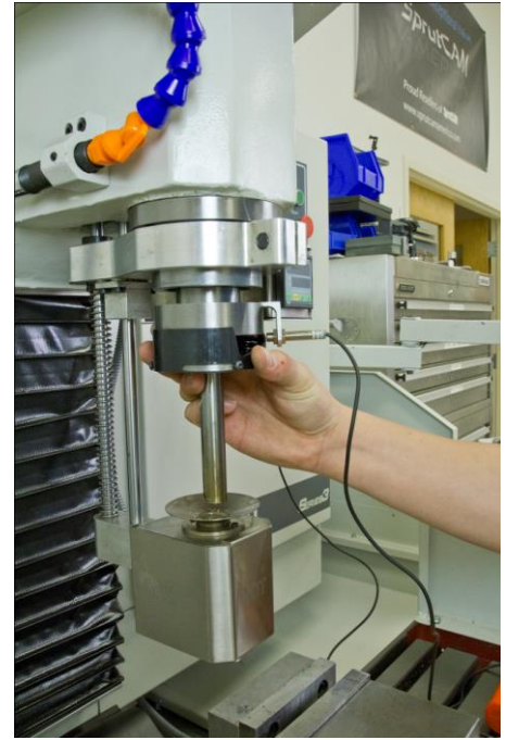
Figure 7. Insert Ram as shown. Adjust sensor position to avoid interference.
