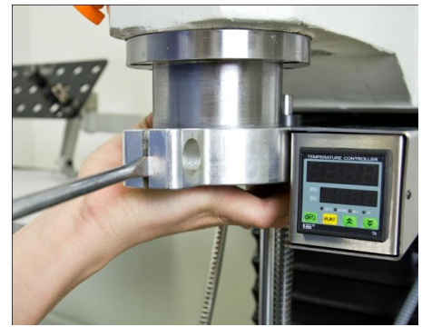
Figure 5. Use a screw driver to pry apart collar if fit is too tight.
