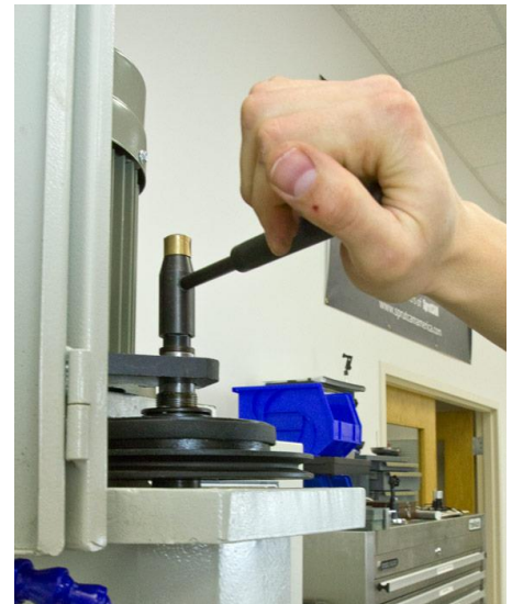
Figure 8. Tighten drawbar to secure the ram.
