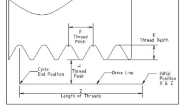
**NOTE:** As G07 Lathe Diameter Mode is always in force, the values for I, J and K are diameter measurements.
