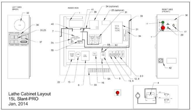
The related power distribution component locations in the electrical cabinet are highlighted in **Figure 8.3**.
