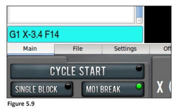
Click the *MDI* field to use the MDI line; the line is highlighted. Type the command, using the *Backspace, Delete, Left* and *Right* arrow keys to correct typing errors. Press *Enter* to execute the command; press *Esc* to abandon it.
