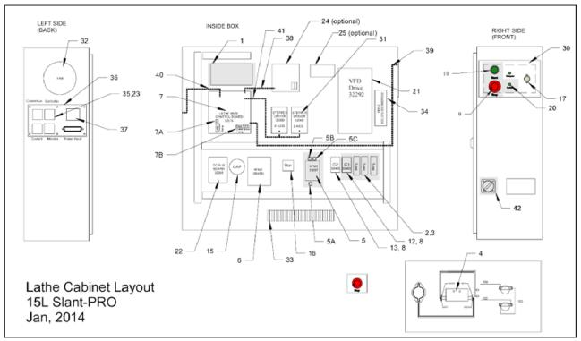
The related control power distribution component locations in the electrical cabinet are highlighted in **Figure 8.5**.
