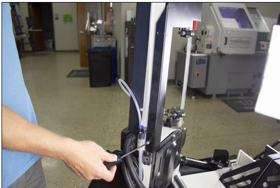
Figure 10-7: Removing the screws securing the blade cover to the bandsaw.
