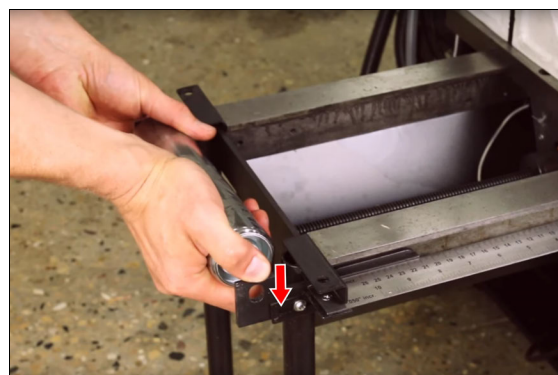
Figure 4-9: Squeezing the spring-loaded post.
