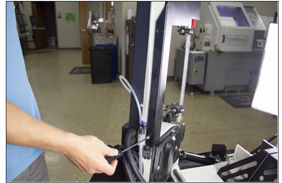
Figure 6-6: Removing the screws securing the blade cover to the bandsaw.
