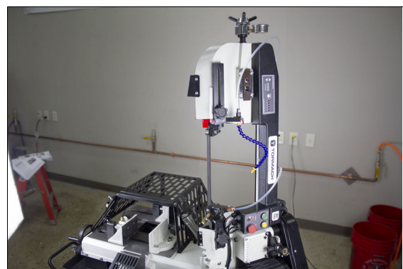
Figure 10-5: Bandsaw head lifted upright.
