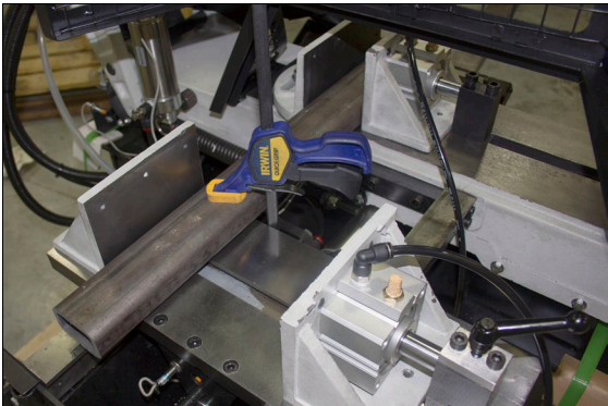
Figure 10-14: Clamp secured to the 24-in. stock.
