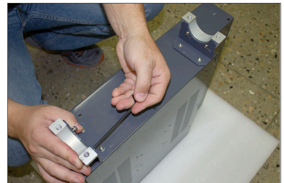
Figure 4-184: Split collars attached to the mount arm brackets on the controller.
