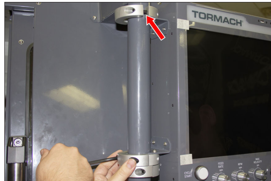
Figure 4-187: Loosely attaching the split collars to the mount arm.
