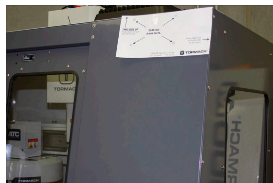
Figure 4-174: Drill template taped to the enclosure.
