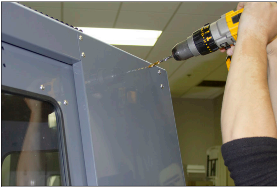
Figure 4-175: Drilling holes into the top of the enclosure.
