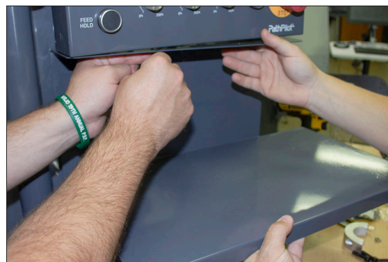
Figure 4-188: Attaching the keyboard tray to the bottom of the controller.
