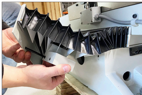
Figure 4-7: Installing the Y-axis bellows spacer.
