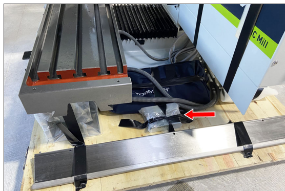
Figure 4-6: Y-axis bellows spacers on the pallet.
