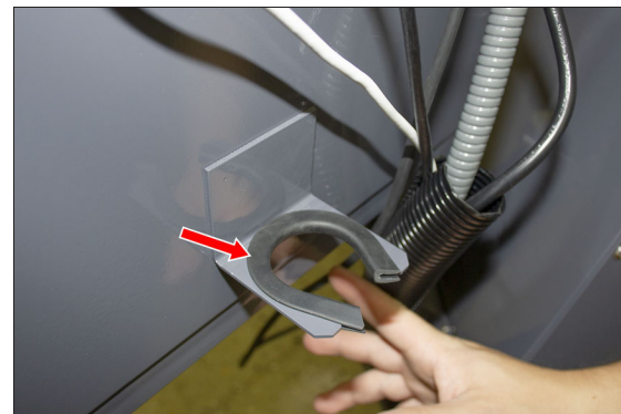
Figure 4-191: Rubber attached to the bracket on the keyboard tray.
