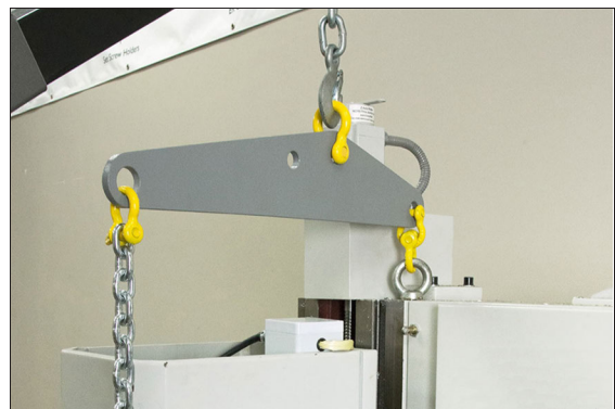
Figure 4-15: Lifting Bar Kit connected to the machine.
