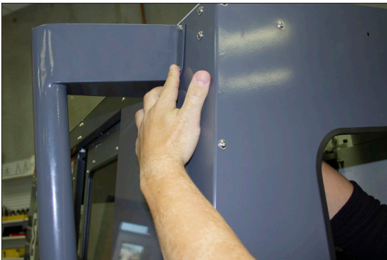
Figure 4-176: Securing the top of the mount arm to the enclosure.
