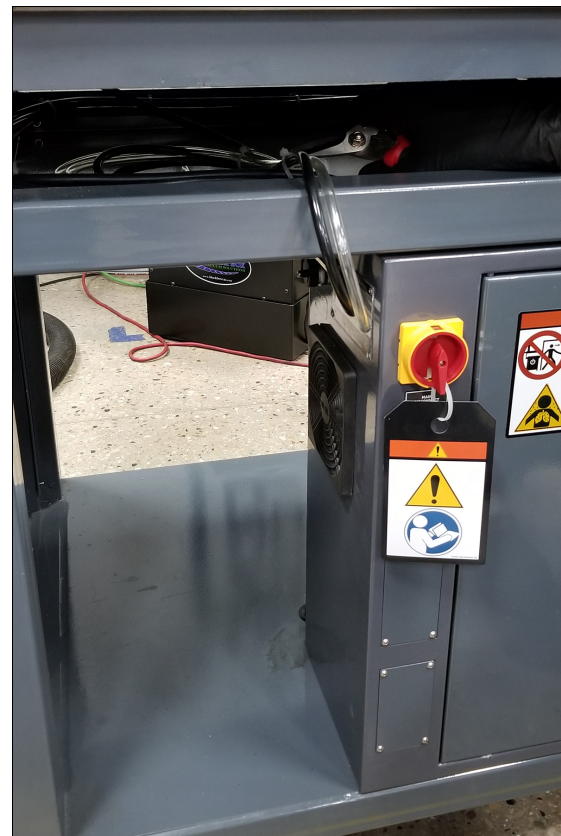
Figure 4-29: The Main Disconnect switch on the side of the machine's electrical cabinet.
