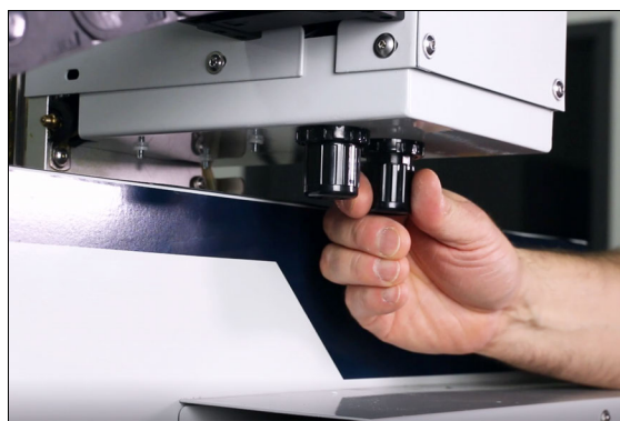
Figure 4-91: Unlocking the dust shoe extend pressure regulator.
