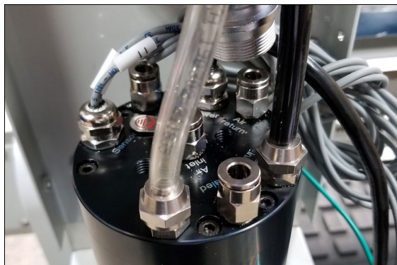
Figure 4-53: Water line connections.
