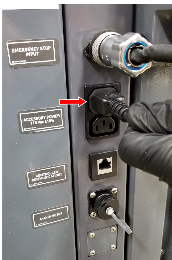
Figure 4-25: Connecting the monitor cable to the Accessory Power Port.
