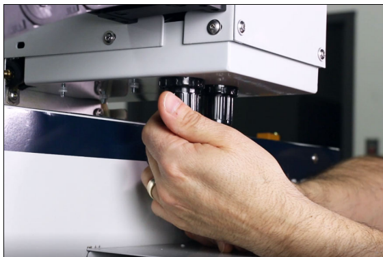
Figure 4-93: Unlocking the dust shoe lift pressure regulator.
