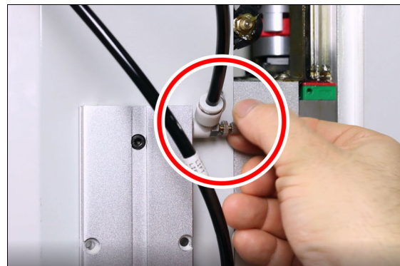
Figure 4-95: Loosening the dust shoe lift speed control valve.
