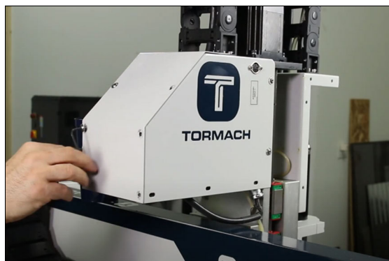
Figure 4-56: Rear Z-axis access panel.
