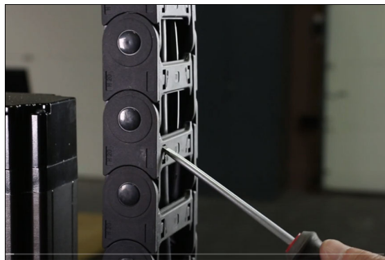
Figure 4-55: Removing pieces of the energy chain.
