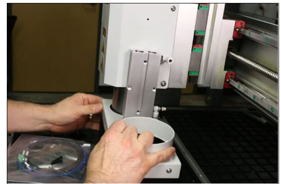
Figure 4-74: Sliding the dust shoe onto the spindle.
