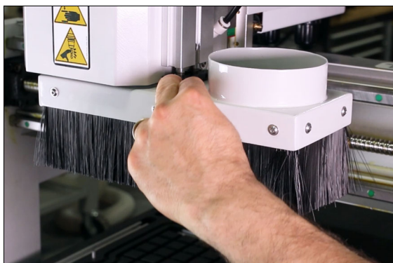
Figure 4-94: Pressing down on the dust shoe.
