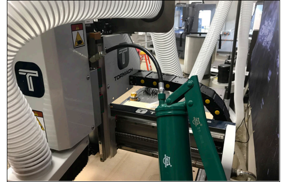
Figure 10-6: Lubricating a remote-mounted lubrication port with the Grease Gun.
