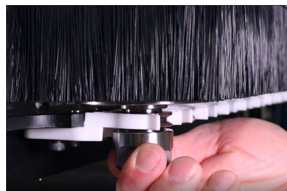
Figure 4-101: Rotating the tool holder to feel when the drag increases.
