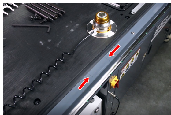
Figure 4-82: Linear rail cover punch-outs.
