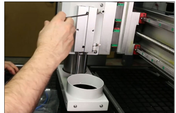
Figure 4-75: Mounting the dust shoe onto the spindle cover.
