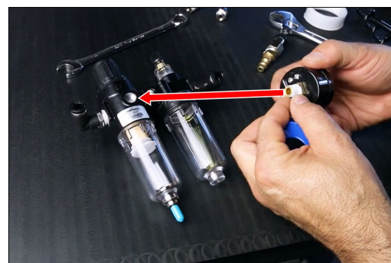
Figure 4-67: Preparing the dial for installation on the FRL.
