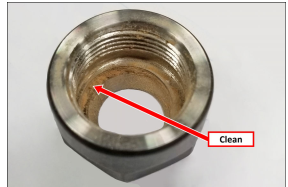
Figure 10-1: Example of a collet nut with dust and resin buildup.
