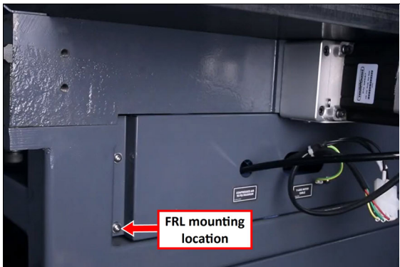
Figure 4-68: Hex screw to remove for mounting the FRL.
