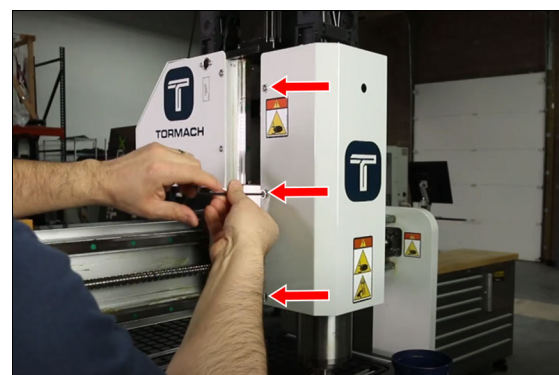
Figure 4-45: Removing the M5 screws that secure the front spindle cover.
