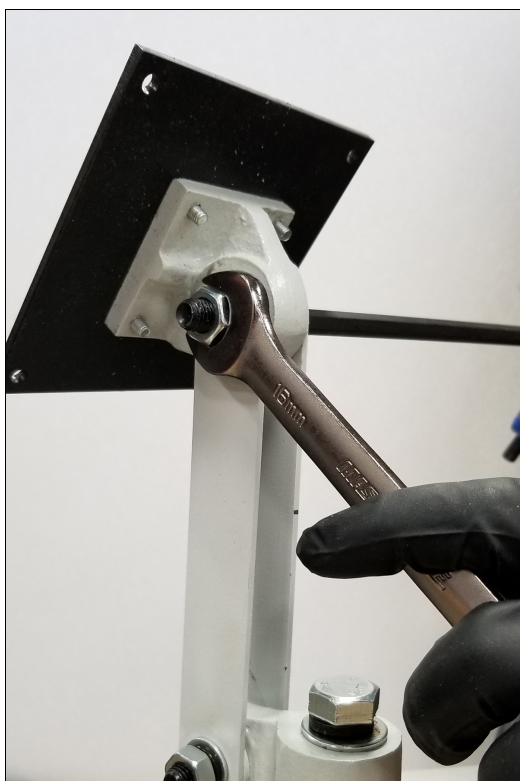
Figure 4-12: Tightening the monitor bracket in place.
