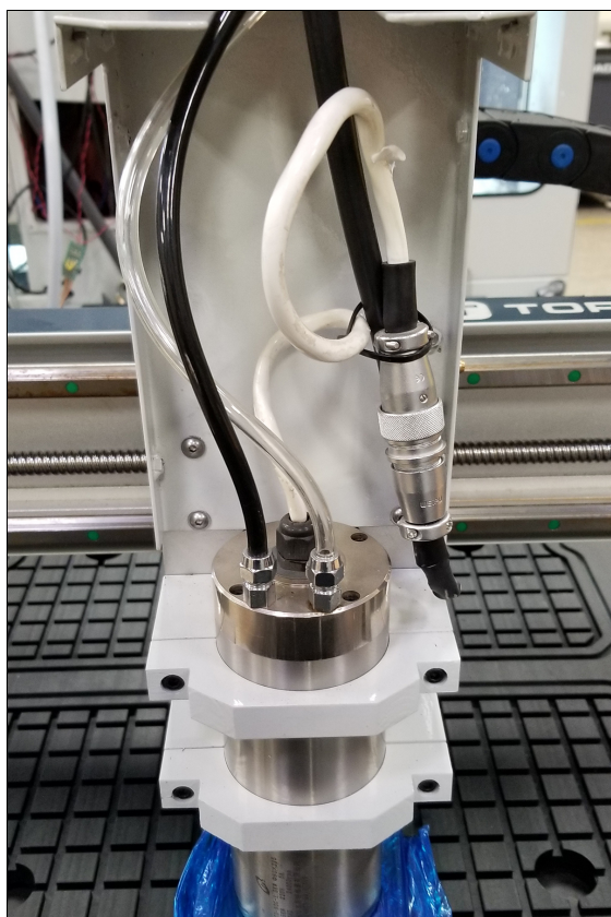
Figure 4-46: Spindle power connector.
