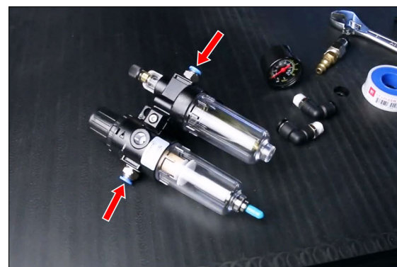
Figure 4-65: Preinstalled push-to-connect fittings on the FRL.
