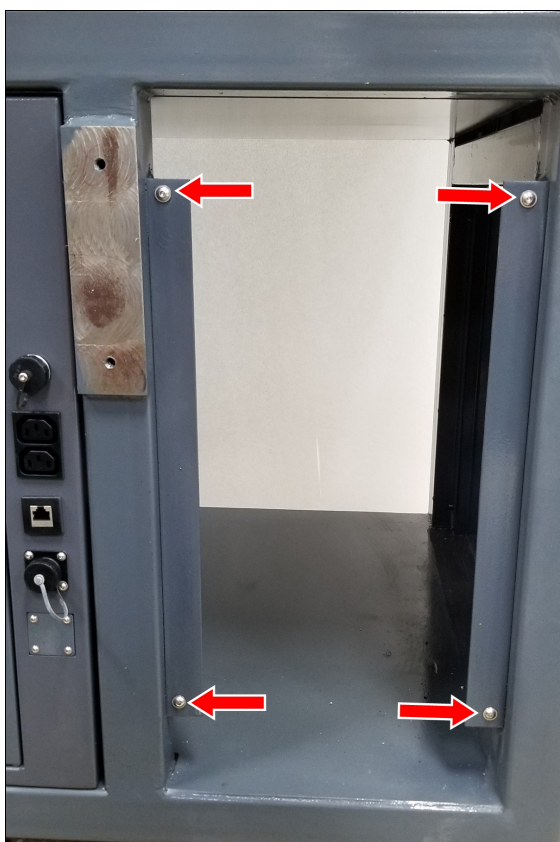
Figure 4-7: Stand end panel hardware installed on the machine stand.
