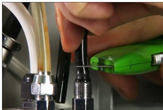
Figure 4-48: Cutting the water lines from the fitting.
