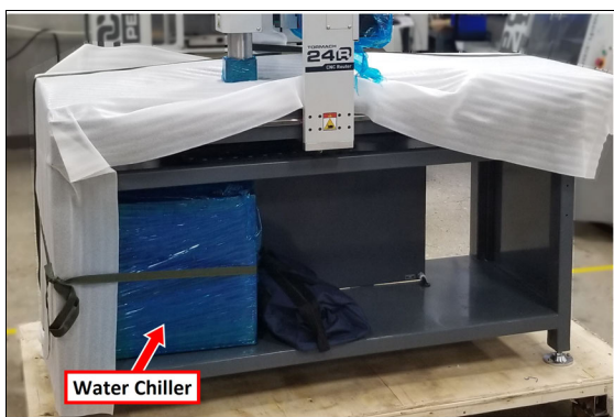
Figure 4-1: Water chiller packaged for shipping inside of the machine stand.
