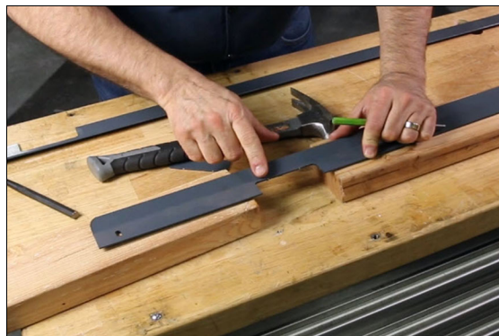
Figure 4-85: Linear rail cover with punch-out removed.
