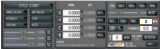
Figure 7-94: Spindle RPM DRO field.
