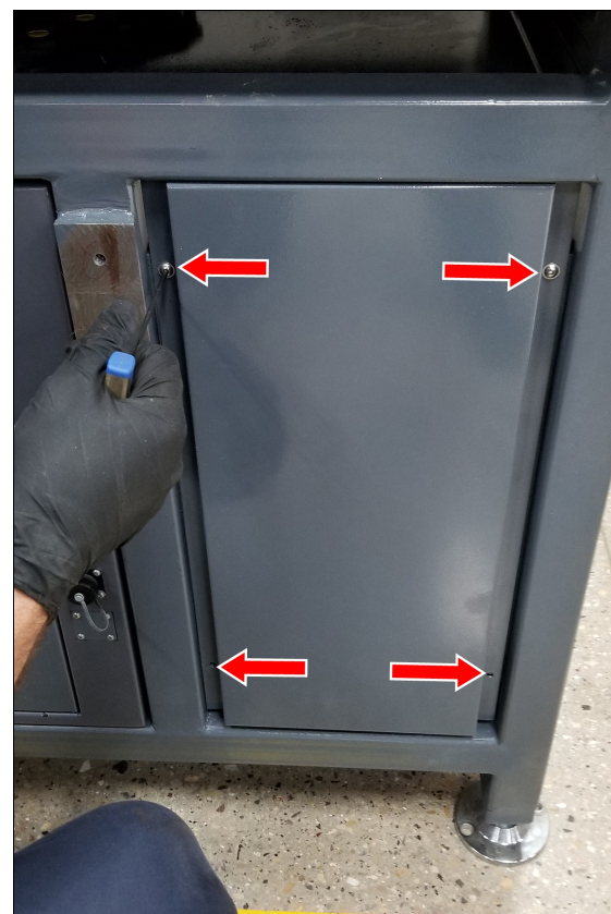
Figure 4-8: Installing the stand end panel on the machine stand.
