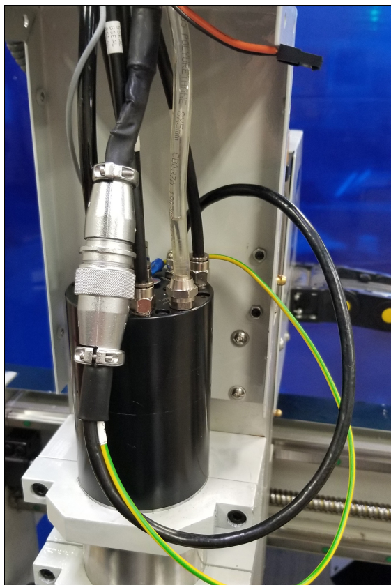
Figure 4-54: Spindle power connector.
