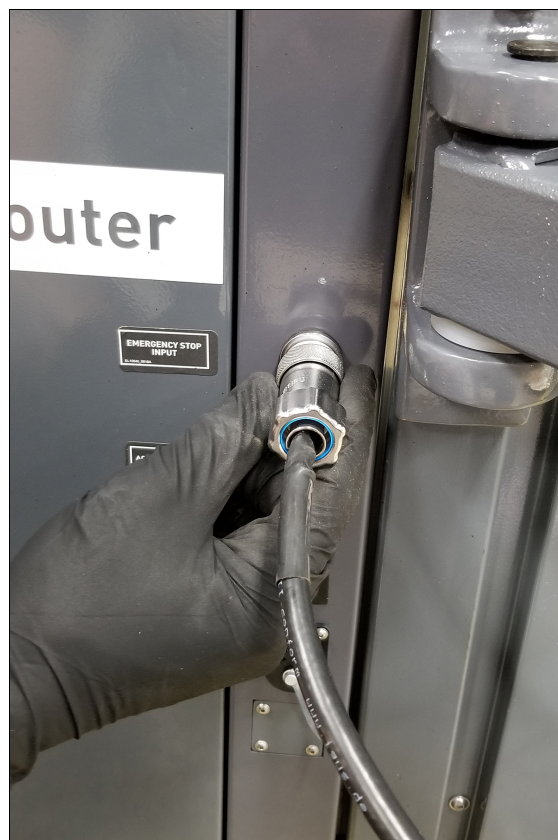
Figure 4-23: Operator box cable connected to the Emergency Stop Input port.
