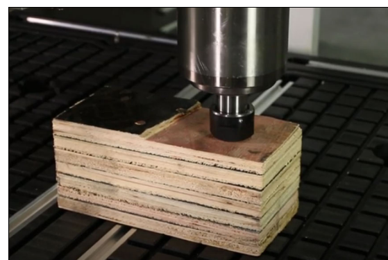
Figure 4-44: Wood block to support the spindle.
