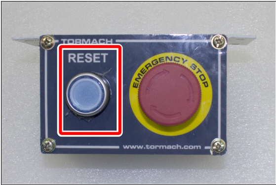
Figure 4-32: The Reset button on the operator box. The axis drives are now powered on.
