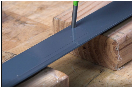
Figure 4-84: Using a punch to break the tab closest to the edge of the linear rail cover.
