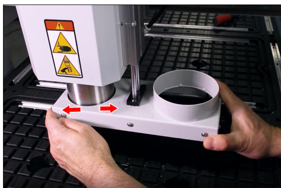
Figure 4-76: Adjusting the position of the dust shoe.
