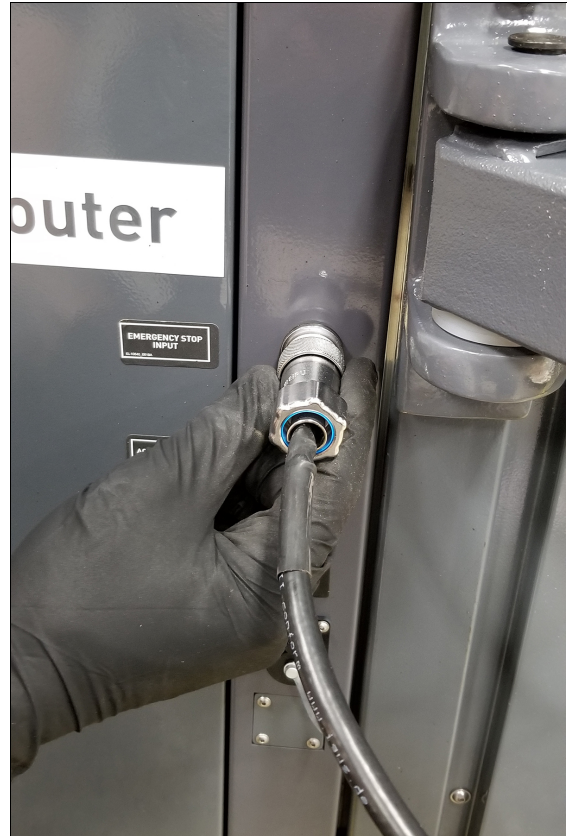
Figure 4-15: Operator box cable connected to the Emergency Stop Input port.
