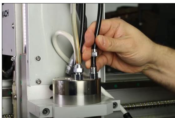
Figure 4-47: Two water lines on the existing spindle.
