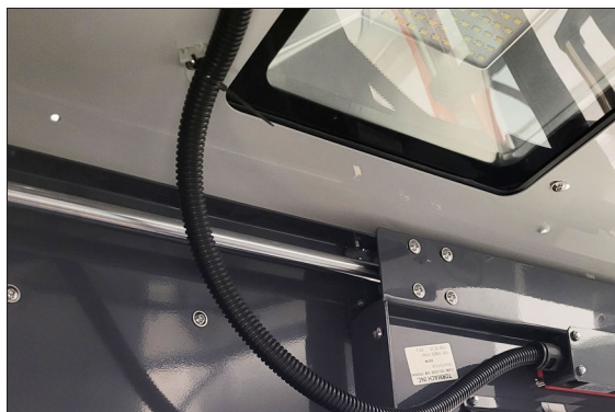
Figure 4-131: Cable routing from the enclosure light to the door, without interference.
