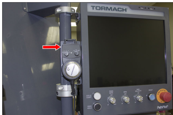
Figure 4-156: Jog pendant on the front of the console assembly.
