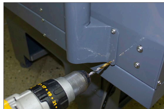
Figure 4-145: Drilling the remaining three holes into the enclosure.
