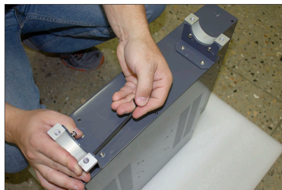
Figure 4-151: Split collars attached to the mount arm brackets on the controller.
