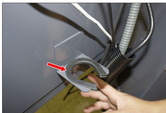
Figure 4-158: Rubber attached to the bracket on the keyboard tray.
