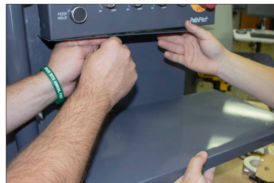
Figure 4-155: Attaching the keyboard tray to the bottom of the controller.
