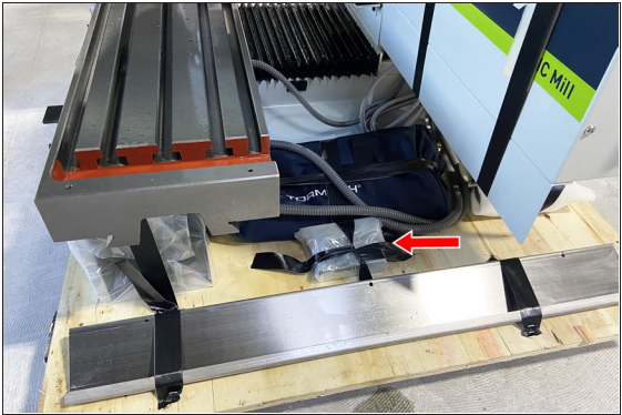
Figure 4-6: Y-axis bellows spacers on the pallet.
