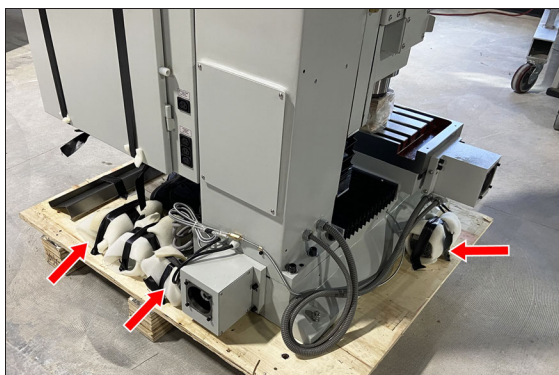
Figure 4-8: Axis motors secured to the pallet.
