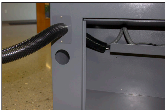
Figure 4-162: Access panel attached to the machine stand.
