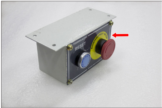
Figure 4-37: Example of the Emergency Stop button locked in the disabled position.
