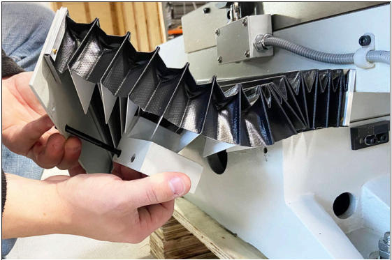
Figure 4-7: Installing the Y-axis bellows spacer.
