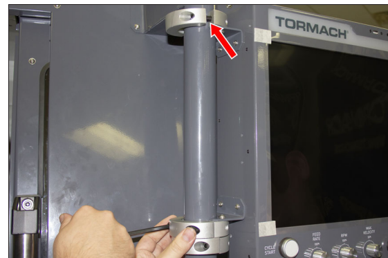
Figure 4-154: Loosely attaching the split collars to the mount arm.
