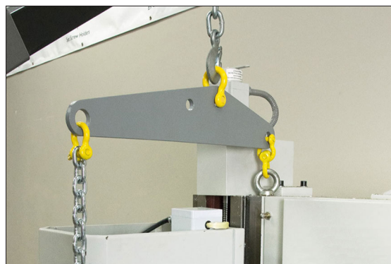
Figure 4-18: Lifting Bar Kit connected to the machine.
