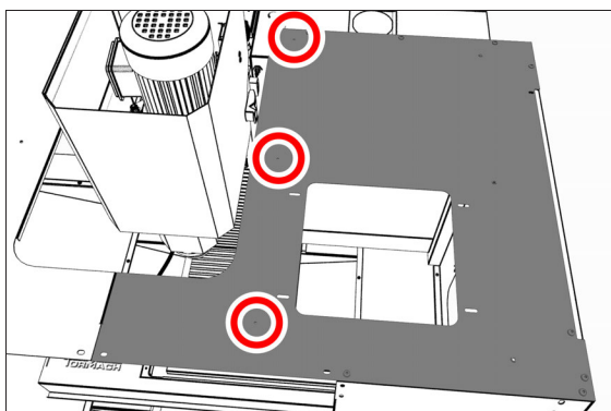
Figure 4-97: Location to attach three cable tie anchors.
