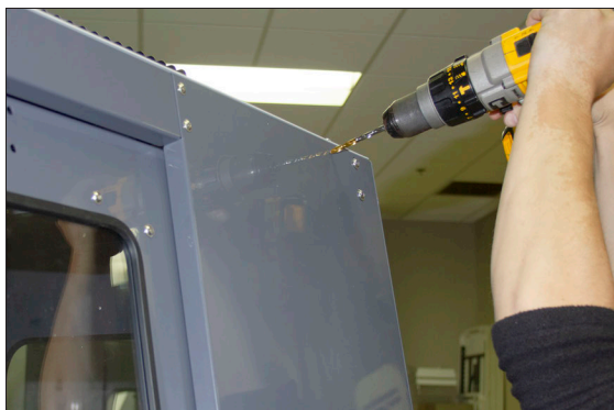
Figure 4-142: Drilling holes into the top of the enclosure.
