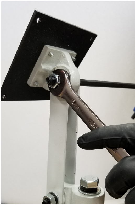
Figure 4-25: Tightening the monitor bracket in place.
