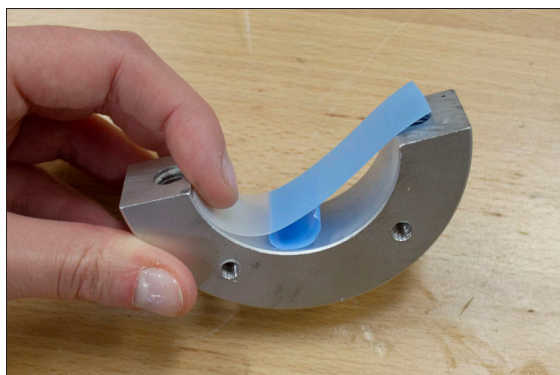
Figure 4-148: Adhering tape on the inside of a split collar.
