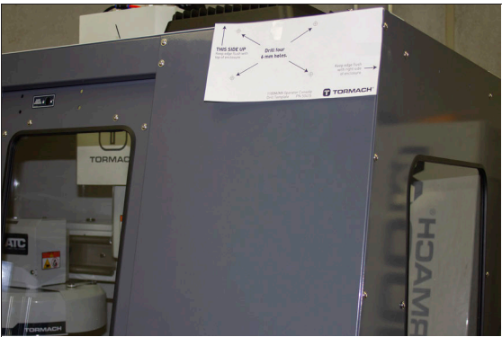
Figure 4-141: Drill template taped to the enclosure.
