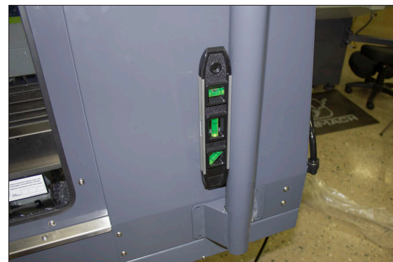
Figure 4-137: Bottom of the mount arm level on the enclosure.
