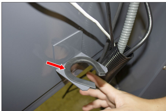
Figure 4-151: Rubber attached to the bracket on the keyboard tray.
