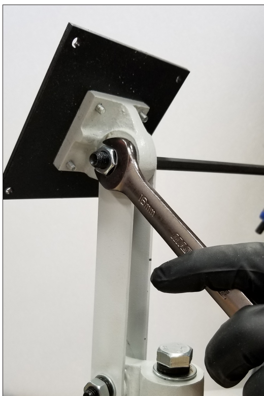
Figure 4-18: Tightening the monitor bracket in place.
