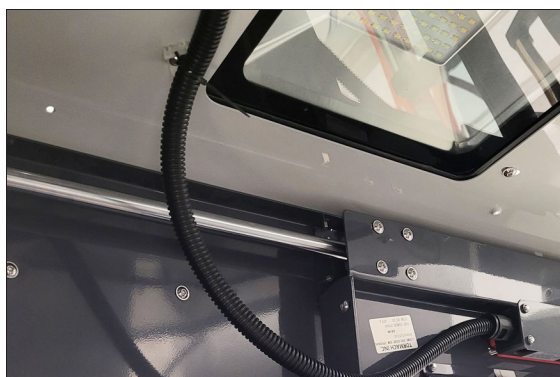
Figure 4-124: Cable routing from the enclosure light to the door, without interference.
