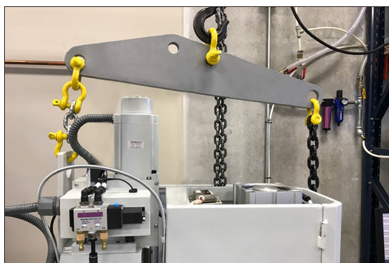
Figure 4-12: Lifting Bar Kit connected to the machine.
