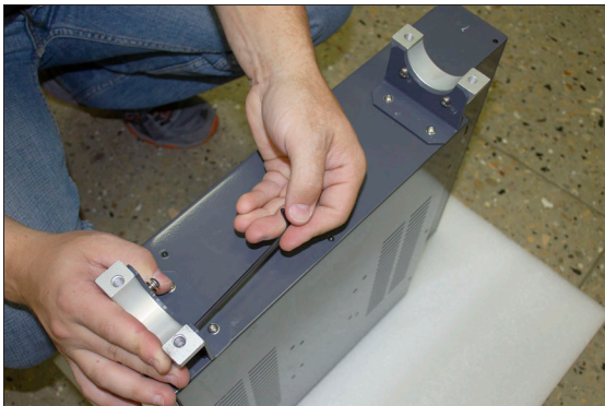
Figure 4-144: Split collars attached to the mount arm brackets on the controller.
