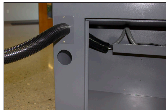
Figure 4-155: Access panel attached to the machine stand.
