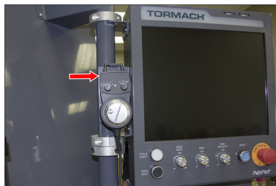
Figure 4-149: Jog pendant on the front of the console assembly.
