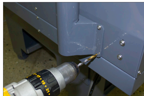
Figure 4-138: Drilling the remaining three holes into the enclosure.
