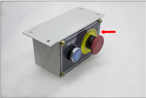
Figure 4-30: Example of the Emergency Stop button locked in the disabled position.
