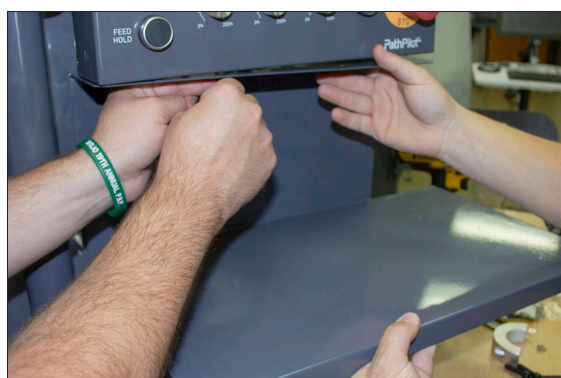
Figure 4-148: Attaching the keyboard tray to the bottom of the controller.
