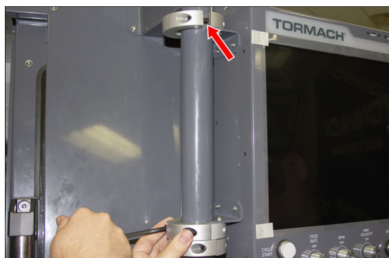
Figure 4-147: Loosely attaching the split collars to the mount arm.
