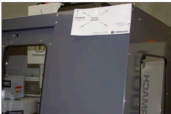
Figure 4-134: Drill template taped to the enclosure.
