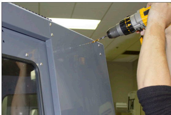
Figure 4-135: Drilling holes into the top of the enclosure.
