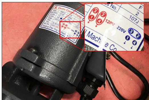
Figure 4-45: Coolant pump motor jumper configuration diagram.
