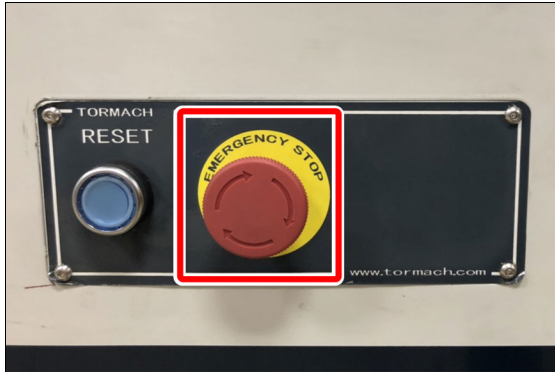
Figure 4-23: The Emergency Stop button on the operator box.
