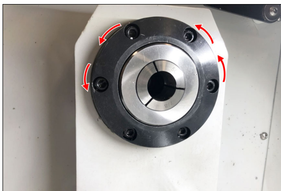
Figure 4-35: Spindle rotating counterclockwise, in the correct forward direction.
