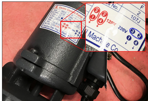
Figure 4-46: Coolant pump motor jumper configuration diagram.
