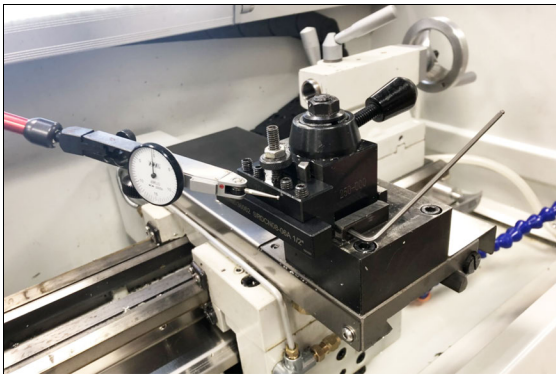
Figure 4-42: Magnetic dial test indicator on the face of the tool holder.
