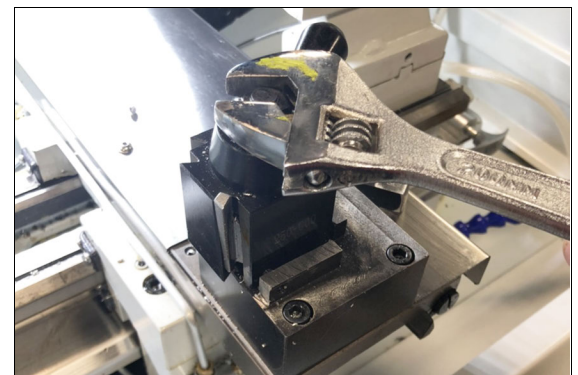
Figure 4-44: Tool post nut securely tightened with an adjustable wrench.
