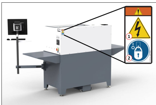
Figure 1-1: Example of a safety decal on the electrical cabinet door.
