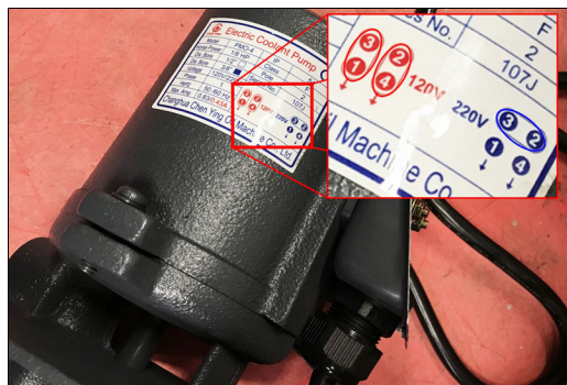
Figure 4-46: Coolant pump motor jumper configuration diagram.
