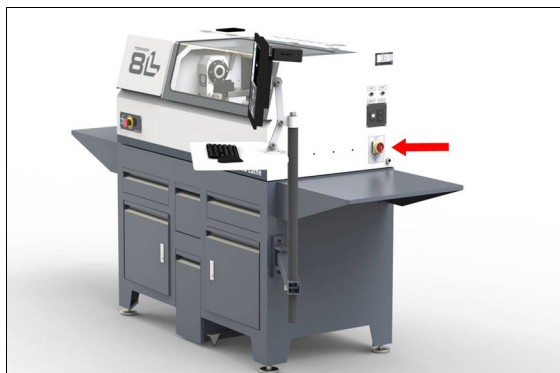
Figure 4-21: The Main Disconnect switch on the side of the machine's electrical cabinet.
