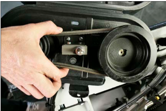
Figure 4-16: Testing the tension of the motor belt.
