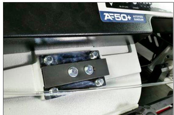
Figure 10-10: Socket head cap screws used to adjust the blade tracking.
