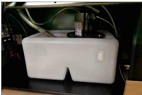
Figure 4-4: Coolant hose installed into the coolant tank.
