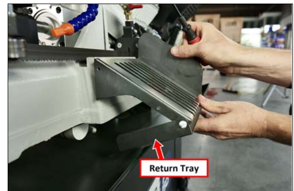
Figure 4-13: Outfeed guide correctly aligned.
